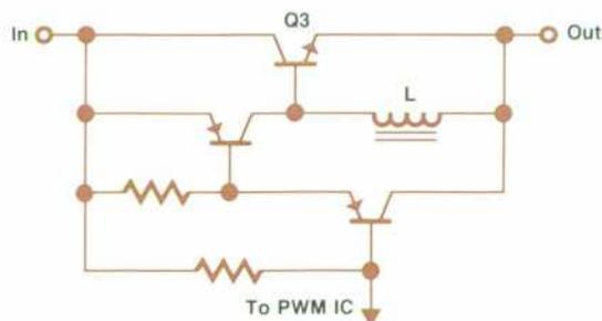
Fig. 3. Turn on/off circuit for the V2 and V3 regulators. Energy stored in the inductor turns Q3 off rapidly to reduce storage time and improve efficiency.
