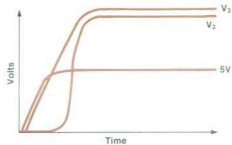
Fig. 4. Turn-on sequencing is designed for proper operation of semiconductor memory devices.
