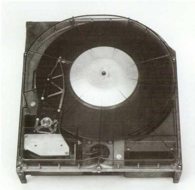
**Fig. 1.** This 12-megabyte fixed disc provides built-in mass memory for the HP 300 Computer.
