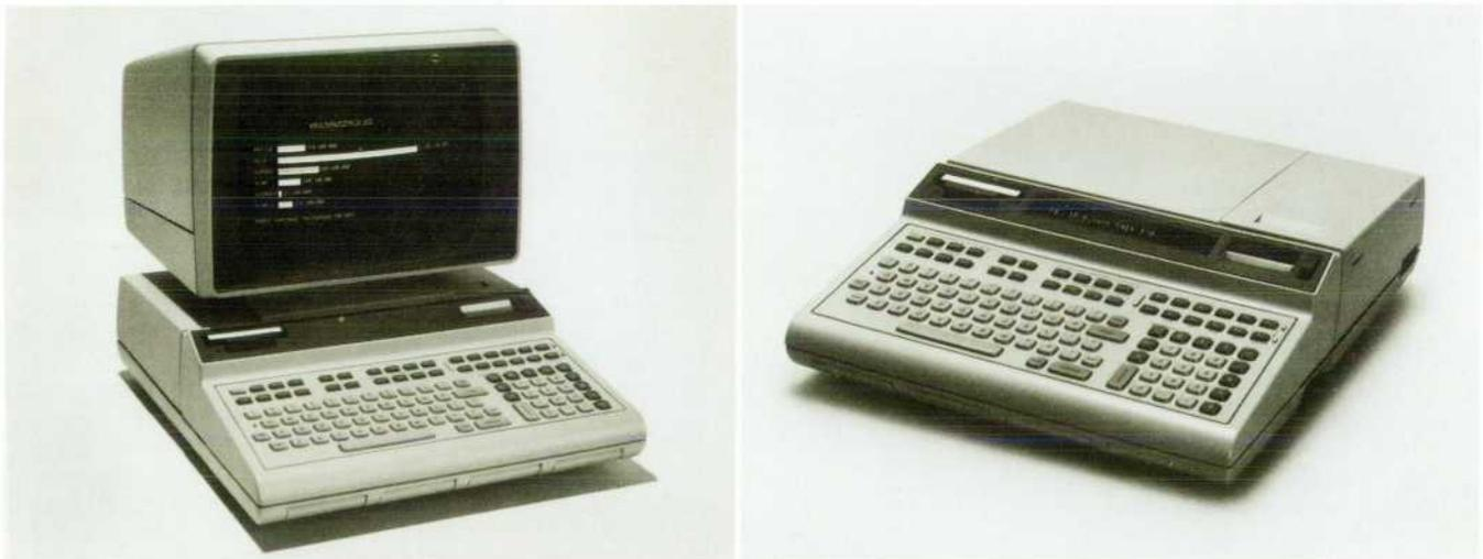
**Fig. 1.** Model 9835A/B Desktop Computer's large memory capacity and powerful I/O system make it especially well suited for control and data acquisition applications in addition to scientific computation. Model 9835A has a 24-line CRT display. Model 9835B has a single-line display.
