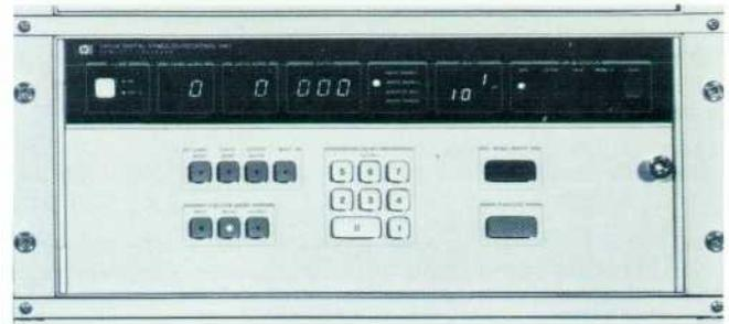
Fig. 5. Front panel of the digital stimulus/response unit.
