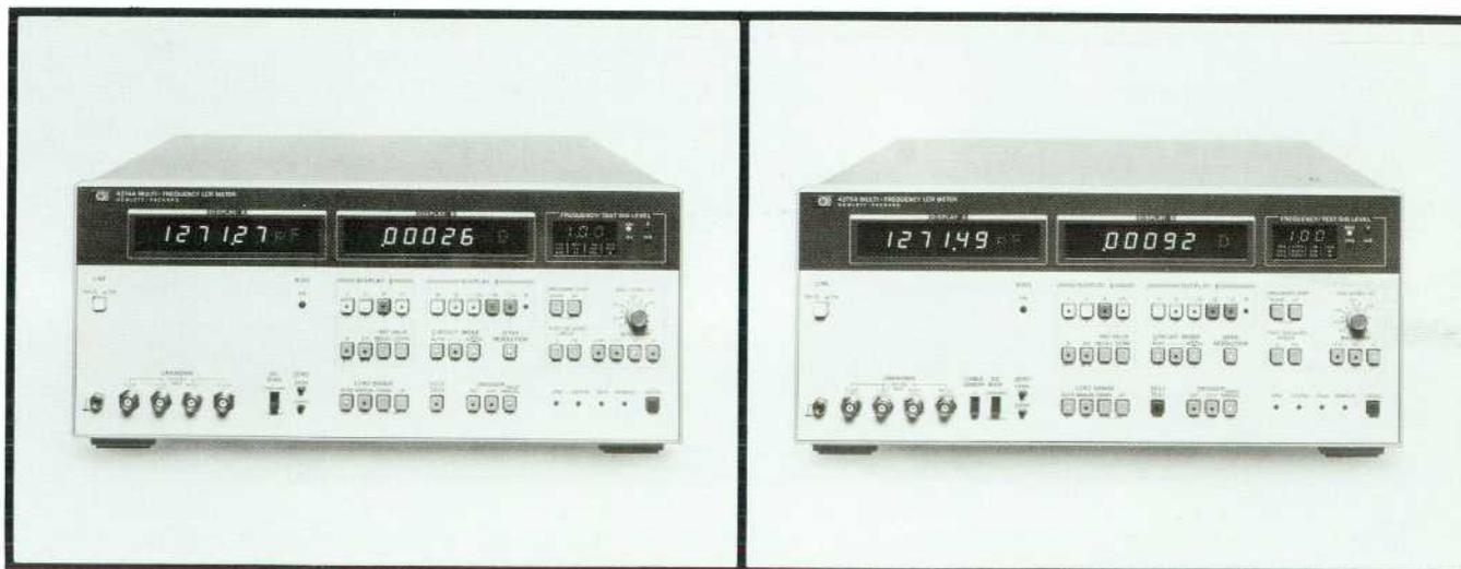
**Fig. 1.** Models 4274A (l) and 4275A (r) Multi-Frequency LCR Meters measure component values and circuit parameters at any of ten standard frequencies and two optional frequencies. Test signal levels and dc bias levels are also selectable. Model 4274A covers a frequency range of 100 Hz to 100 kHz while Model 4275A covers 10 kHz to 10 MHz. Both instruments have 4½-digit displays and can provide 5½-digit readouts in their high-resolution modes.
