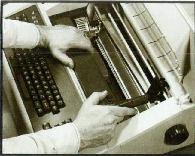
Fig. 6. Full-width ribbon cartridge is easily replaced.
