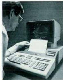
**Cover:** Model 9845A Desktop Computer, also called System 45, incorporates several often-needed peripheral devices, including a CRT with both alphanumeric and graphics capability, mass storage in the form of two cartridge tape units (one optional), and an optional page-width printer that has graphics capability. Four I/O slots are provided for external peripherals and the HP Interface Bus.
