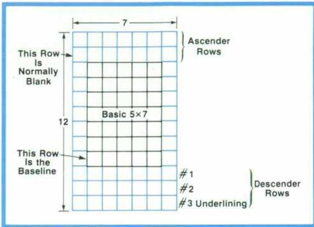
**Fig. 4.** Characters are formed in a basic 5x7-dot matrix contained in a field of 7x12-dots. Two columns of dots between each character are not used in the alphanumeric mode, but are used in the graphics mode to form continuous plots.
