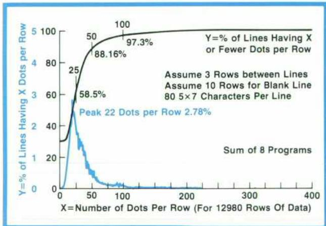
**Fig. 5** Results of a study of the number of dots per row in a typical listing shows that 88% of the rows have 50 dots or fewer. To reduce peak power demand, the printer is designed to burn at most 56 dots at a time. Thus a complete 560-dot line takes ten burn sequences.
