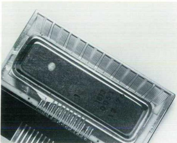
**Fig. 1.** In previous printheads used only for alphanumeric printing there are spaces between groups of print resistors that correspond to the two-dot space between characters. These spaces were used for the return path for the resistor current.
