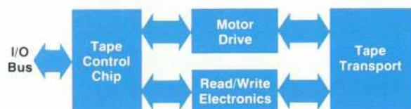
**Fig. 1.** System 45 tape control system. The tape control chip is a new 14,000-transistor NMOS design.
