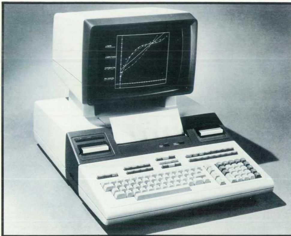
**Fig. 1.** The new HP Series 9800 System 45 features the most powerful central processor and the largest built-in mass memory now available in a desktop computer. It also has a 12-inch CRT display, enhanced BASIC language, an optional graphics package with high-speed hard-copy printing, and applications software.
