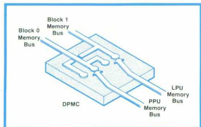
**Fig. 4.** Dual-port memory control (DPMC) coordinates memory accesses by the two processors. When the LPU and the PPU must communicate with the same block of memory the DPMC switches between them at a 50% duty cycle.
