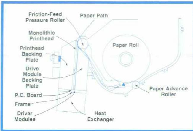
Fig. 2. Sectional view of the printhead/paper relationship.
