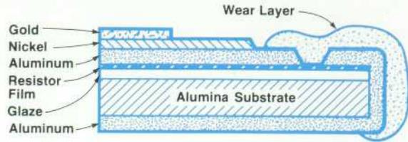
**Fig. 4.** Cross-section of the thin-film System 45 printhead.
