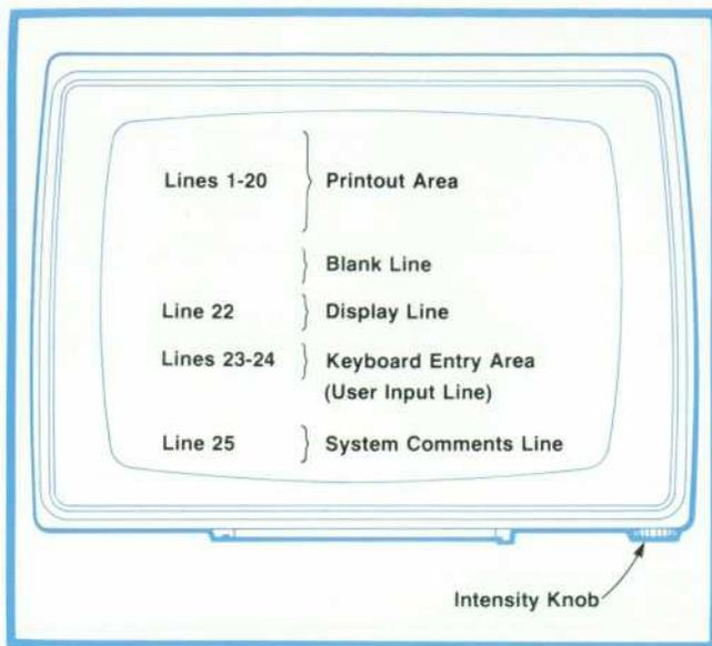
**Fig. 2.** Most keyboard operations are immediately reflected in the display. In the normal mode, the display is divided into a printout area for program-generated information and an interaction area that handles communications between the user and the computer.
