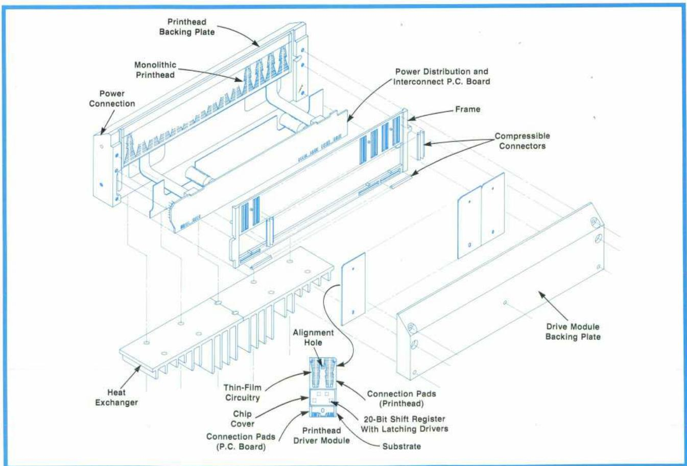
**Fig. 1.** Exploded view of the printhead of System 45's optional built-in thermal printer. 560 print resistors are selectively energized to darken the thermal paper where information is to be recorded.
