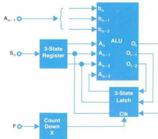
**Fig. 4.** Implementation of the divide-by- $F$  function.
