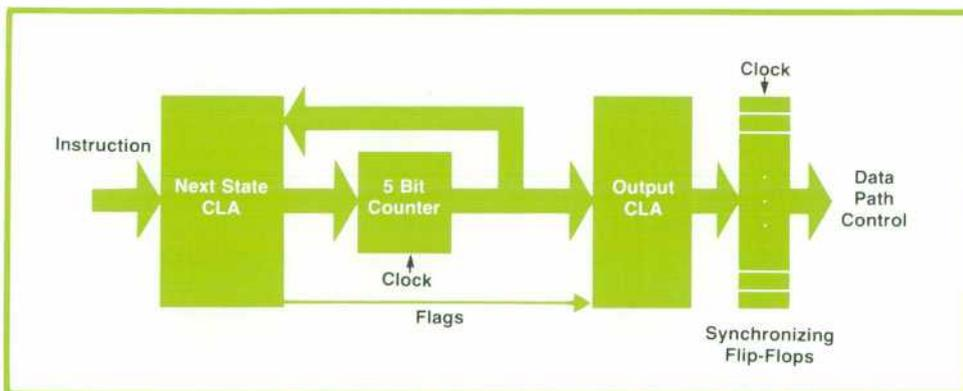
**Fig. 8.**  $MC^2$  control section block diagram. Custom logic arrays (CLAs) are like programmable logic arrays (PLAs, a form of read-only memory) but do not have a full output matrix. The CLAs are controlled by a five-bit counter.
