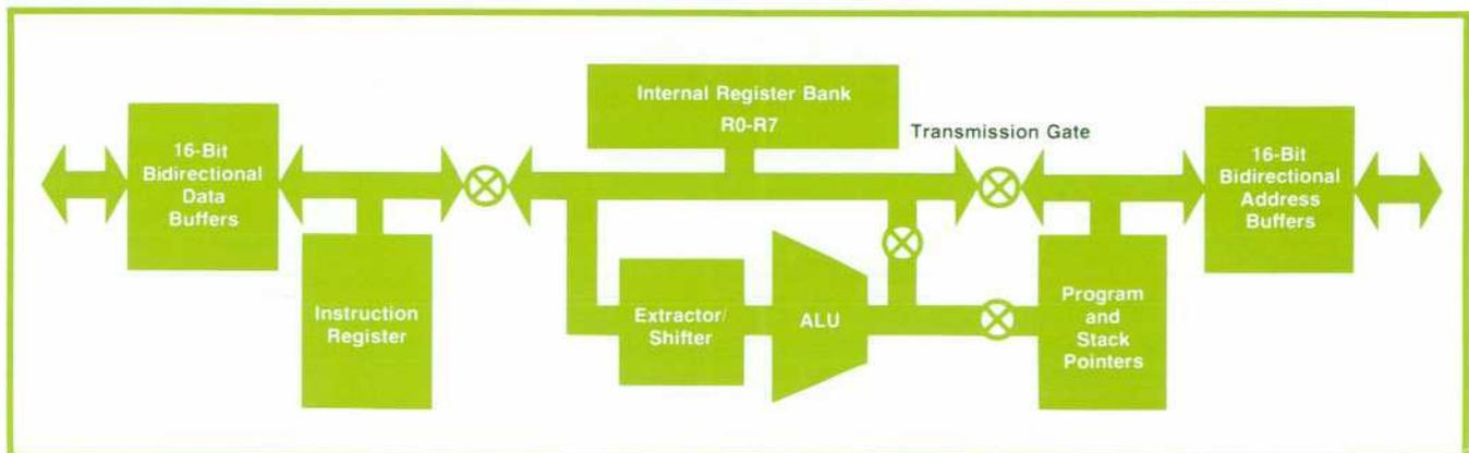
**Fig. 5.** MC<sup>2</sup> data path block diagram. External registers used for I/O operations are treated in the same way as the internal registers. This allows flexibility in manipulating data while keeping the length of instructions to a minimum.
