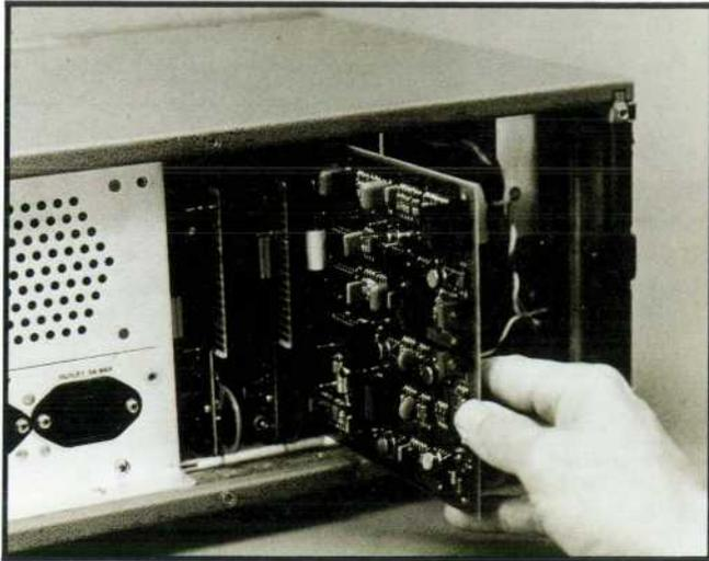
**Fig. 2.** Adding another monitoring technique to the Model 8030A Cardiocograph is simply a matter of inserting a circuit card and then using the corresponding transducer. The instrument automatically makes the necessary circuit connections for whatever transducer is in use.
