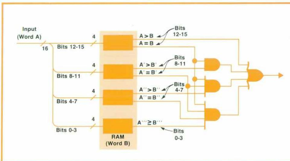
**Fig. 9.** A multi-bit comparator for wide digital numbers is implemented with relatively few components using the technique of Fig. 8b.
