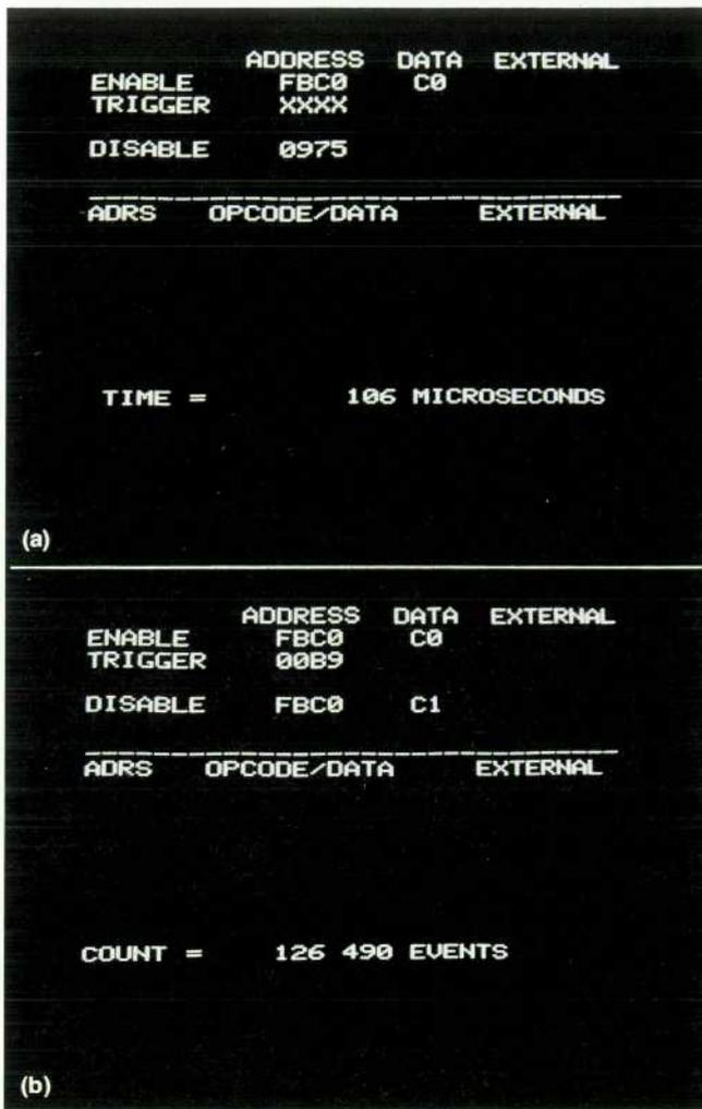
**Fig. 5.** When operating in the TIME INTERVAL mode (a), Model 1611A measures the execution time from one point in a program (selected by TRIGGER ENABLE) to another point (TRIGGER DISABLE). In the COUNT TRIGGERS mode (b) the instrument counts the number of times a particular address (00B9) is accessed between ENABLE and DISABLE points, in this case through a loop beginning and ending at address FBC0.
