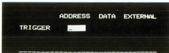
**Fig. 2.** When a TRACE SPECIFICATION key is pressed an inverse video field is created. The black underline in the white field blinks to show where the next character entered will be positioned. When the field is filled or closed by other means, the display automatically reverts to normal video.
