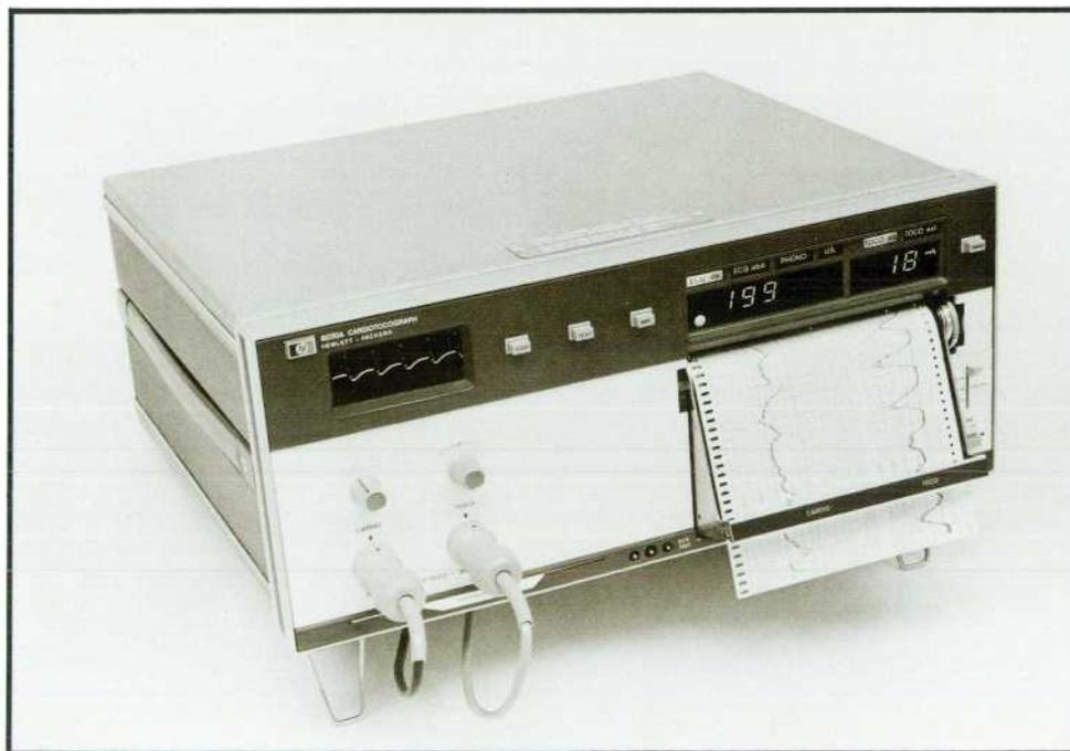
**Fig. 1.** Model 8030A Cardiotocograph monitors fetal heart rate and plots it on its built-in strip-chart recorder along with a plot of labor activity. The instrument can monitor fetal heart rate by any one of four techniques and its design combines this versatility with operating simplicity and compactness.
