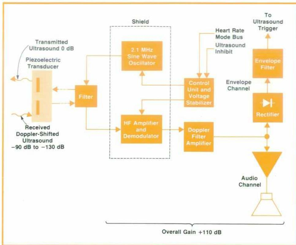
Fig. 6. Simplified block diagram of the ultrasound circuit.
