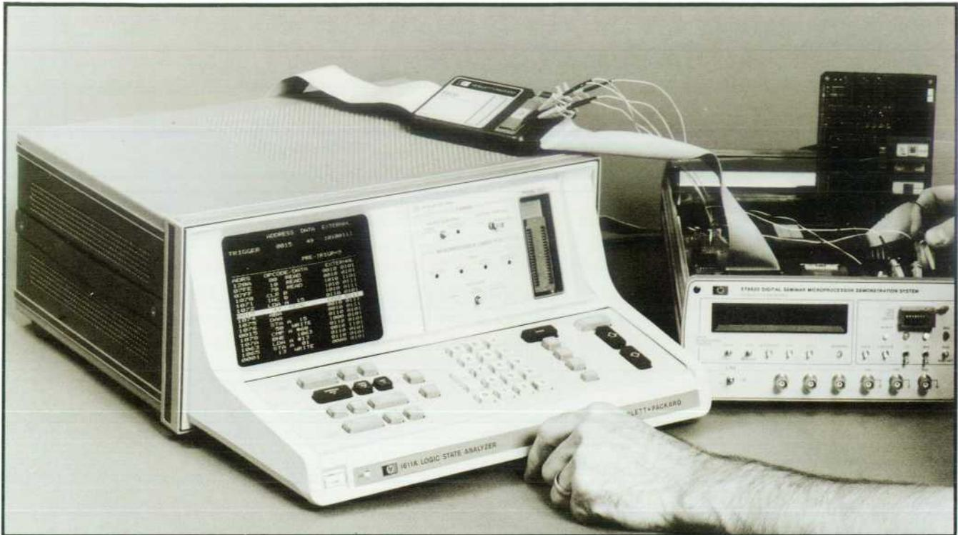
**Fig. 1.** Model 1611A Logic State Analyzer, designed to test systems using popular microprocessors, captures and displays the sequential flow of states on a microprocessor's DATA and ADDRESS busses and at up to eight other nodes selected by the user.
