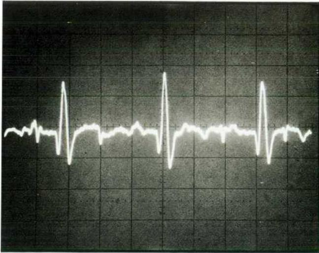
**Fig. 4.** The fetal ECG (small negative peaks) is mixed with the maternal ECG (large peaks) and other interference when sensed by abdominal electrodes. The AECG circuits extract the fetal ECG from the composite signal.
