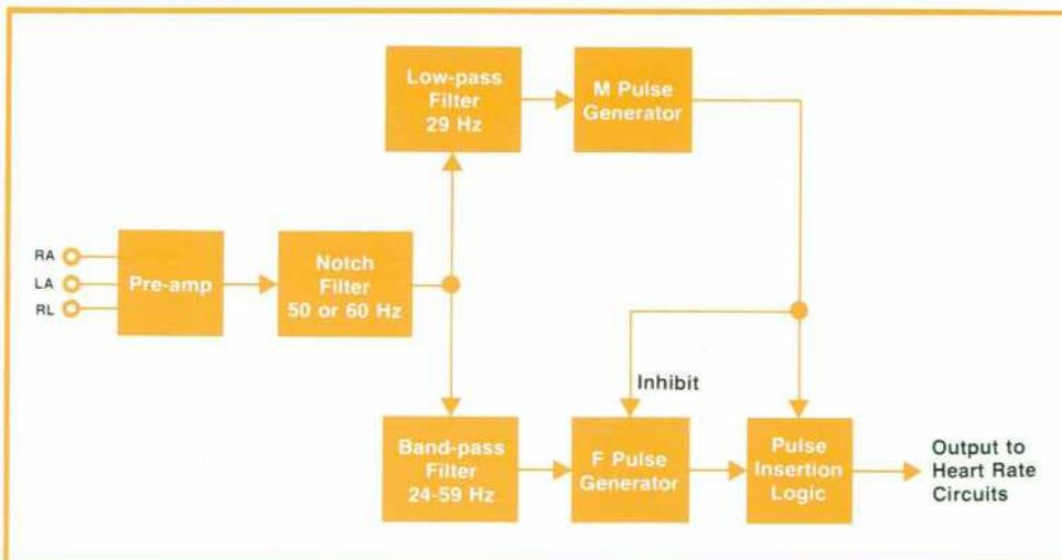
**Fig. 5.** Simplified block diagram of the AECG circuits. The basic scheme is to blank the F channel during a maternal ECG beat so the maternal ECG will not generate an F pulse. If blanking occurs at a time when an F pulse would have occurred, the logic circuits insert a pulse into the output stream.
