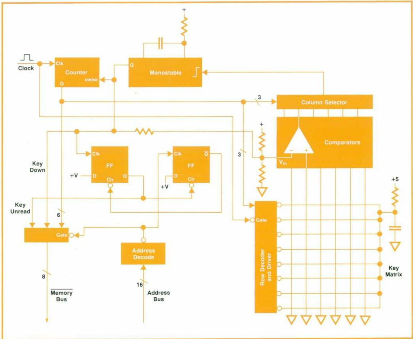
**Fig. 7.** Block diagram of the keyboard scanner. The keyboard is assigned an address in the instrument's memory and is read once every 160  $\mu$ s. The two flags (KEY DOWN and KEY UNREAD) indicate to the instrument's microprocessor whether or not any action should be taken on the 6-bit key code presented to the memory bus.
