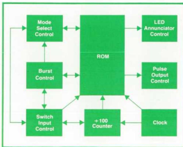
Fig. 3. 546A block diagram. Most circuits are on a single custom IC chip, including the 256-bit ROM.
