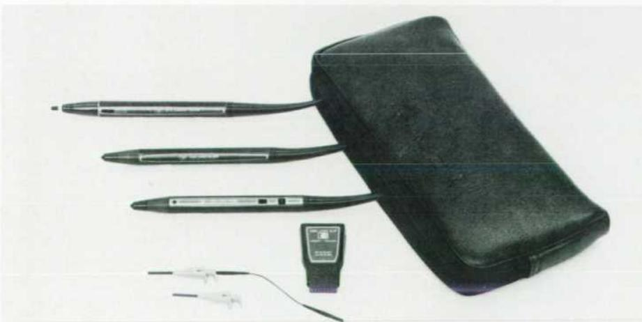
IC Troubleshooting instruments are available in kits consisting of various combinations of logic probe, logic pulser, logic clip, current tracer, logic comparator, and carrying case. Model 5022A Kit (shown) contains the four instruments described in this issue: the 545A Logic Probe, the 546A Logic Pulser, the 547A Current Tracer, and the 548A Logic Clip.
