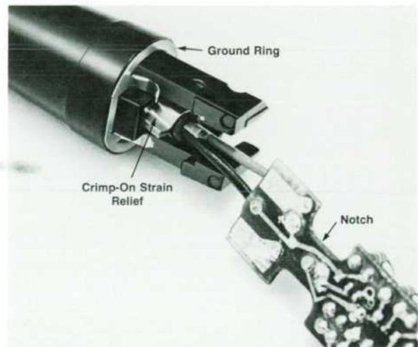
**Fig. 3.** Ground ring provides a ground path from the bottom of the printed circuit board to the end of the extrusion shown in Fig. 2. Crimp-on strain relief pulls back into a cavity and locks the cable into place. Notches in the printed circuit board snap into the rear plastic support for structural rigidity.
