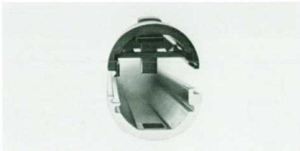
**Fig. 2.** At top is an end view of the upper interlocking extrusion for the 546A Logic Pulsar with the pulser switch in place. Internal slots serve as guides for the sliding switch. Slots in the lower extrusion serve as printed circuit board guides. Lower extrusion is from the 547A Current Tracer, showing the faced and clear alodined end that provides grounding of the case for electromagnetic shielding.
