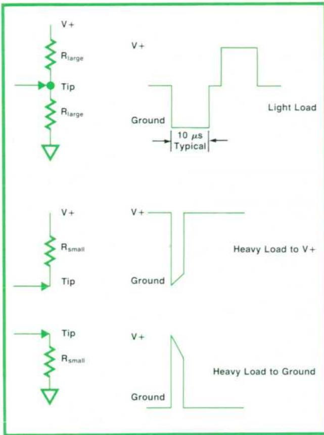
Fig. 5. Typical 546A output waveforms under various loads.
