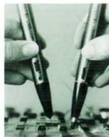
**Cover:** A new troubleshooting team finds many low-impedance faults that elude voltage-sensing instruments. Model 547A Current Tracer (right) reveals the presence and relative size of current steps by the brightness of its built-in lamp.
