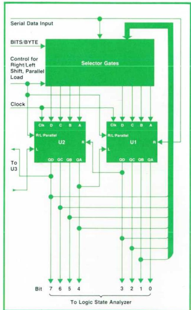
**Fig. 3.** Block diagram of part of the bidirectional shift register. U1 and U2 are commercial IC 4-bit shift registers (U3 is the next IC in the 16-bit shift register chain). The selector gates enable serial data to be loaded through any bit position during right-shift operation (see text).
