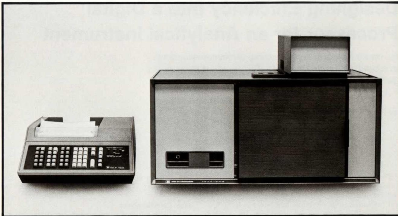
**Fig. 2.** Operating instructions can be entered by way of the keyboard of the new Model 5840A Gas Chromatograph, then edited and recorded on a magnetic strip for later re-entry (Fig. 3). With 30% more memory than Model 5830A, Model 5840A can be programmed to change operating conditions between runs to accommodate sample-to-sample differences.
