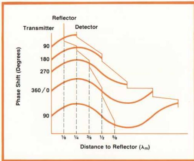
**Fig. 3.** The total station measures distance by measuring the phase shift between the modulation envelopes of two light beams. One is a reference light beam and the other is a light beam that has traversed the unknown distance and been reflected back to the instrument.
