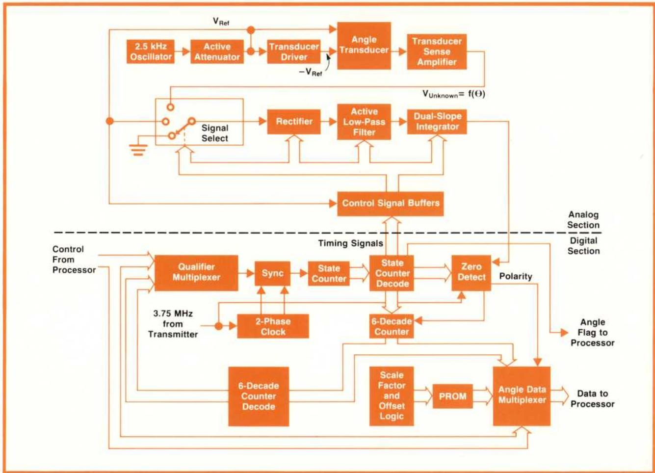
**Fig. 6.** Total station zenith-angle measuring circuits. The analog section excites the angle transducer and converts its output to a dc level that is measured by the dual-slope integration technique. The digital section provides timing and control.
