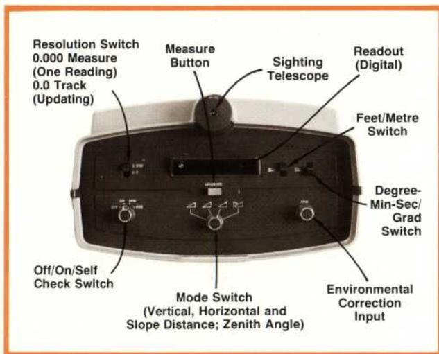
**Fig. 2.** 3810A control panel. Operator simply selects the function and units, aims the instrument at the target point using the integral telescope, and presses the MEASURE button. He can also select a single reading with full resolution or a continuously updated readout with reduced resolution.
