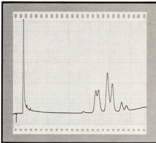
**Fig. 4.** Relatively simple chromatogram made by a manually operated gas chromatograph. To analyze results, the chemist must derive the time delay between sample insertion (marked by the negative spike at left) and each peak, and the area bounded by each peak and the baseline. Special calculations determine areas of peaks that overlap, like those shown here. Chromatograms of complex mixtures such as crude oil may be 10 times as long and have hundreds of peaks.
