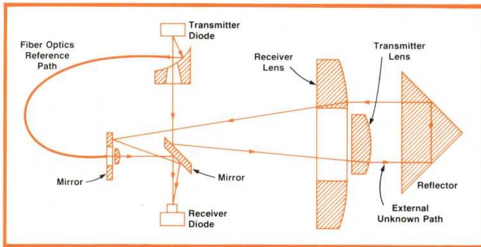
**Fig. 11.** Total station optical system produces a beam angle of 3 arc-minutes. Alignment of transmitter and receiver diodes is carefully done to assure accuracy of  $\pm(5 \text{ mm} + 10 \text{ ppm})$ .
