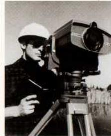
**Cover:** With its built-in calculator, angle transducer, and modulated-light-beam distance measuring system, this one instrument, Model 3810A Total Station, gives the operator a direct readout of distance to a pole-mounted retroreflector held by his rod man. The displayed horizontal distance, corrected for refraction and the earth's curvature, is automatically derived from slope distance and vertical angle.
