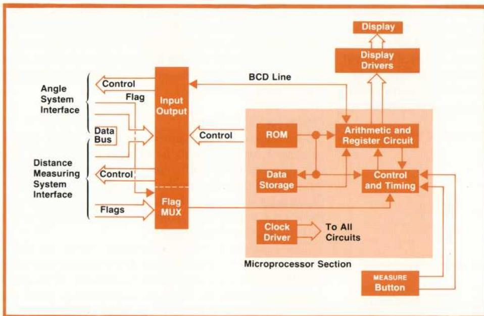
Fig. 9. The microprocessor provides sophisticated control and computational capabilities. This simplified diagram shows the microprocessor and its interfaces to the angle and distance circuits.
