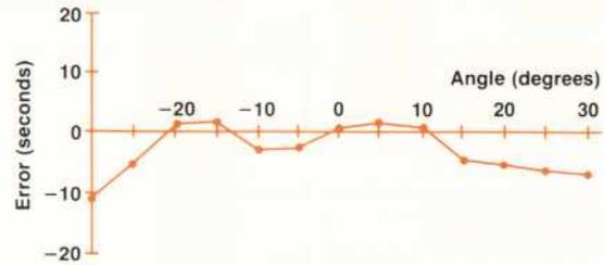
**Fig. 2.** Typical linearity error of vertical angle transducer
