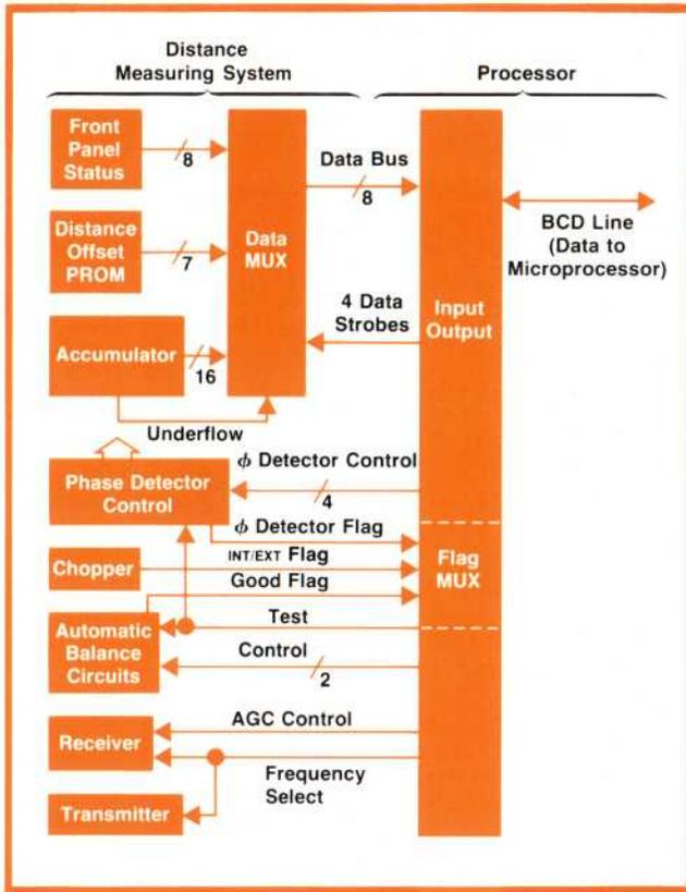
**Fig. 10.** A more detailed look at the interface between the microprocessor and the distance measuring circuits. In a distance measurement the processor handles all control and computation functions, including statistical analysis of the raw data to detect marginal measuring conditions.
