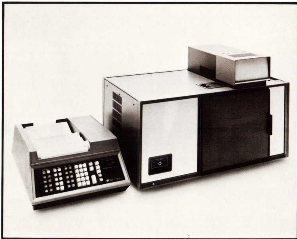
**Fig. 1.** Model 5830A Reporting Gas Chromatograph has a built-in digital processor that operates the instrument throughout an analytical run following instructions entered through the keyboard. It also monitors the detector output, identifying sample components and computing their concentrations, and generates a chromatogram that includes a complete analytical report.
