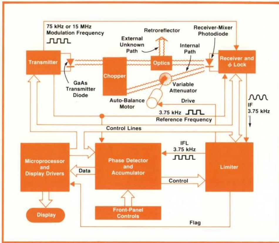
**Fig. 5.** Total station distance measuring circuits. Light at a wavelength of 910 nm is produced by a GaAs diode. The accumulator counts 15-MHz pulses for 100 cycles of the 3.75-kHz reference, first for the internal path and then for the external path; it then holds the average over 100 cycles of the phase difference between internal and external paths. This is transferred to the microprocessor for analysis and display.
