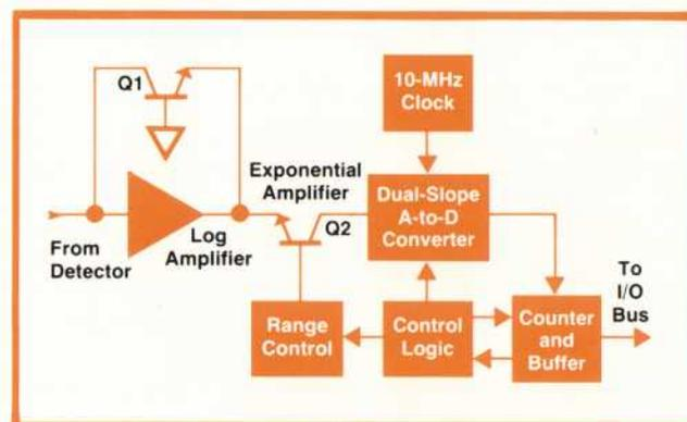
**Fig. 9.** The electrometer for the FID uses the exponential relationship between the emitter-base voltage and collector current of a transistor. In the feedback path of the input amplifier, it derives a logarithmic relationship between input and output (Q1). In the next stage (Q2), it linearizes the amplifier output. Ranging is accomplished by changing the base voltage, and hence the amplification factor, of transistor Q2.
