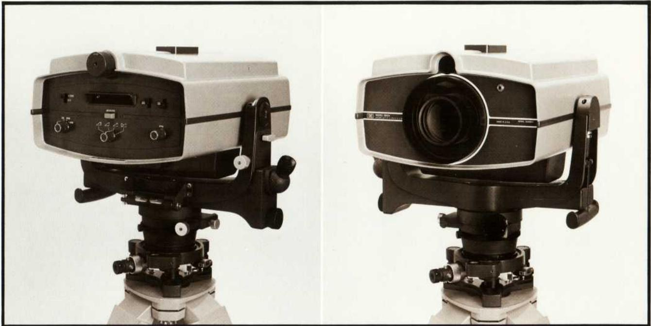
**Fig. 1.** Model 3810A Total Station measures horizontal, vertical, and slope distances and vertical angle, all automatically. Its calibrated base measures horizontal angle. A snap-in battery pod eliminates cables.
