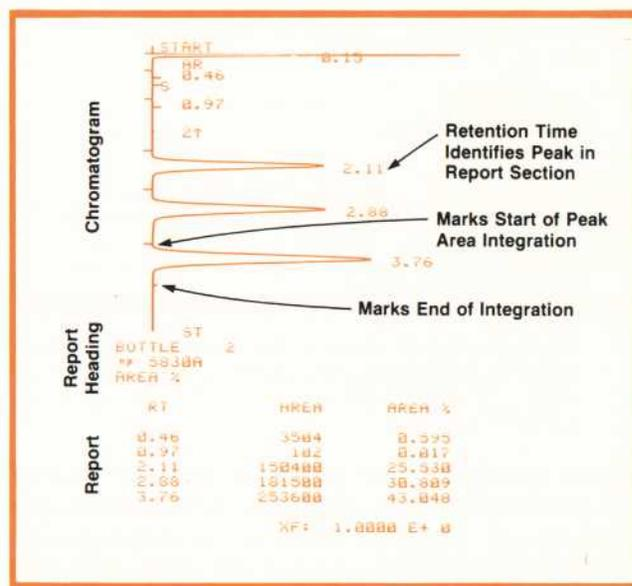
**Fig. 8.** The printer-plotter traces a chromatogram as an analysis proceeds and prints pertinent data on the same sheet of paper. In this example, calculations determine the percentage of each peak with respect to the total area of all peaks. The basic data is retained in memory so the operator can call for additional reports calculated in other ways.
