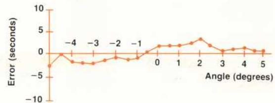
**Fig. 3.** Typical linearity error for small angles
