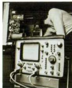
**Cover:** *Display of waveforms fulfills an important function in the world of 1's and 0's just as it always has in the world of analog signals. The oscilloscope pictured here displays waveforms in the traditional manner but it can also be adapted to display 1's and 0's in a data format, as explained in the article beginning on this page.*
