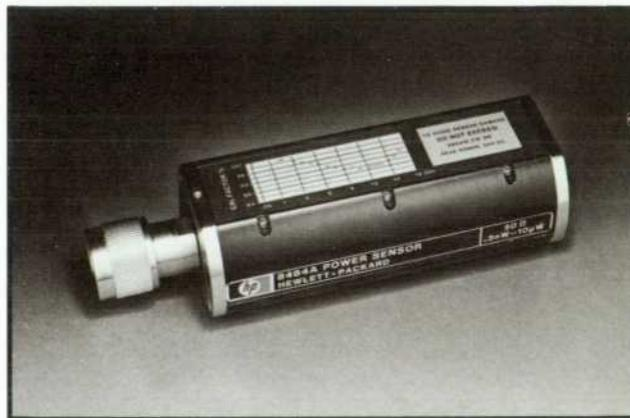
**Fig. 1.** Model 8484A Power Sensor works with HP 435A and 436A Power Meters to measure power from  $-70$  to  $-20$  dBm over a frequency range of 10 MHz to 18 GHz. Calibration factor is shown on housing as a function of frequency.
