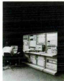
**Cover:** *Test procedures for Hewlett-Packard 9500-Series Automatic Test Systems like this Model 9510D can now be written in ATLAS (Automatic Test Language for Avionics Systems), a high-level language that*
