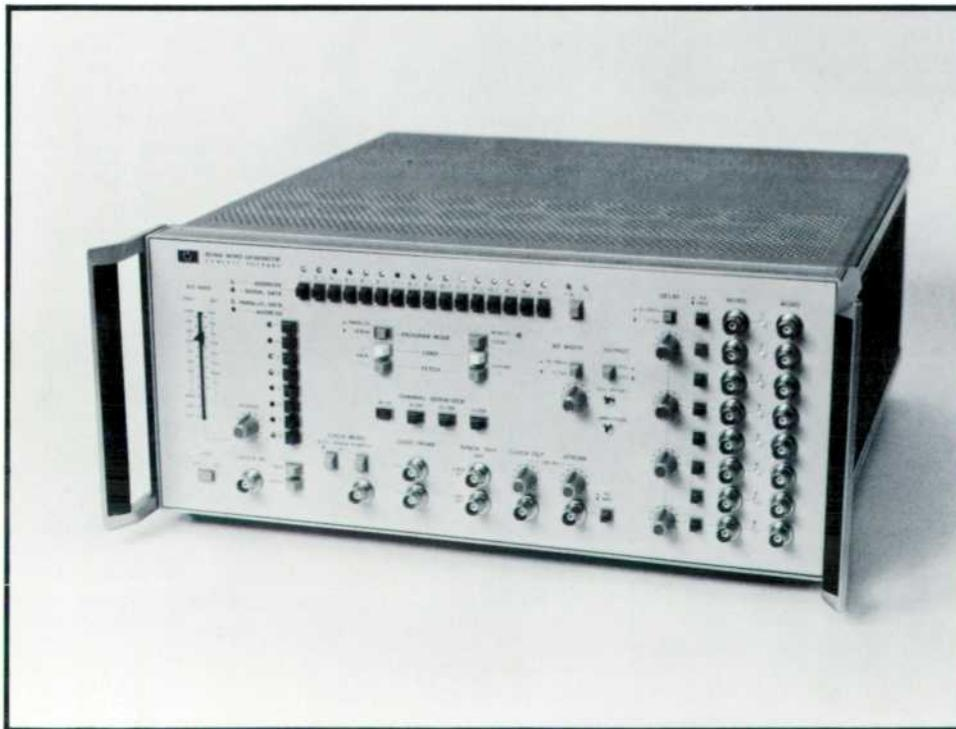
**Fig. 1.** Model 8016A Word Generator has eight output channels, each supplying an independently-selectable 32-bit digital word at bit rates up to 50 MHz. Operator control of the output pulse parameters broadens the range of applications for this instrument.
