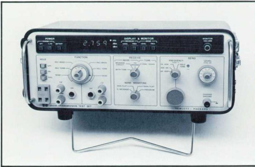
**Fig. 1.** Model 3551A Transmission Test Set makes basic measurements on telephone lines according to North American standards. The front panel is arranged to clarify operation of the instrument. The digital display is autoranged and automatically compensated for the selected impedance.
