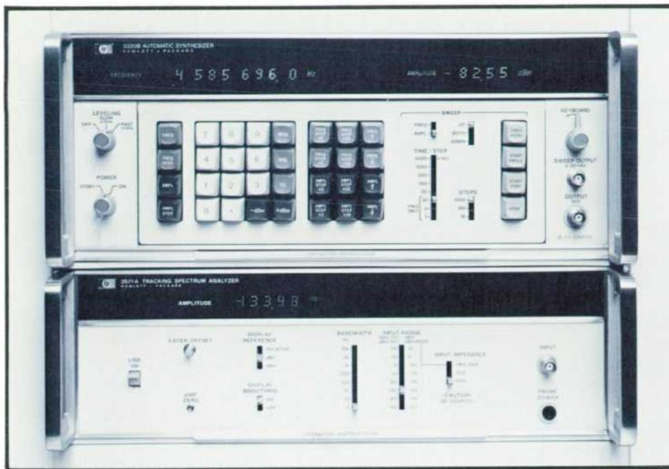
**Fig. 1.** Model 3571A Tracking Spectrum Analyzer (lower unit) works over a 10-Hz-to-13-MHz range using one of the HP synthesizers (upper unit) as a local oscillator. The combination of analyzer and synthesizer is known as the Model 3044A Spectrum Analyzer.
