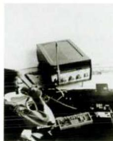
**Cover:** Model 5305A, a new low-cost, compact, portable 1100-MHz frequency counter, is well suited for checking land mobile communications transmitters in two newly opened U.S. channels between 806 and 947 MHz. Its key component, a specially fused, divide-by-four front end, is shown in the foreground. (We are grateful to the mobile paramedic unit of the City of Palo Alto for their help with the background photo.)
