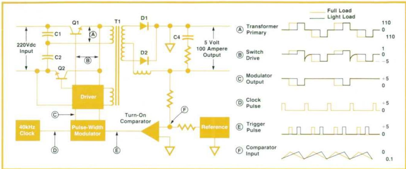
**Fig. 6.** Switching regulator circuit operates at 20 kHz, a repetition rate that is an optimum compromise with respect to cost, size, dissipation, parts availability, and acoustic noise. The colored waveforms show full-load operation. The black waveforms are typical of lightly loaded operation.
