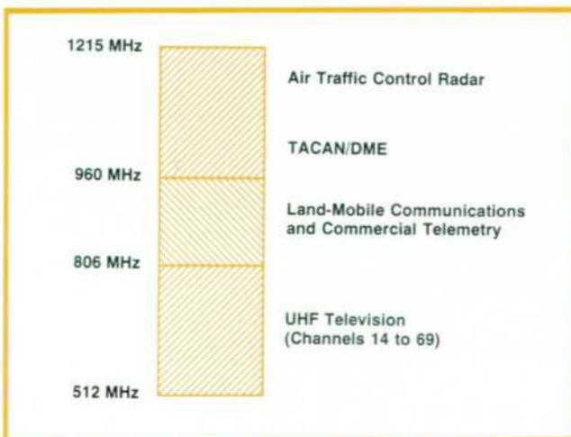
Fig. 2. Frequency spectrum allocations within the range of the 1100-MHz counter.
