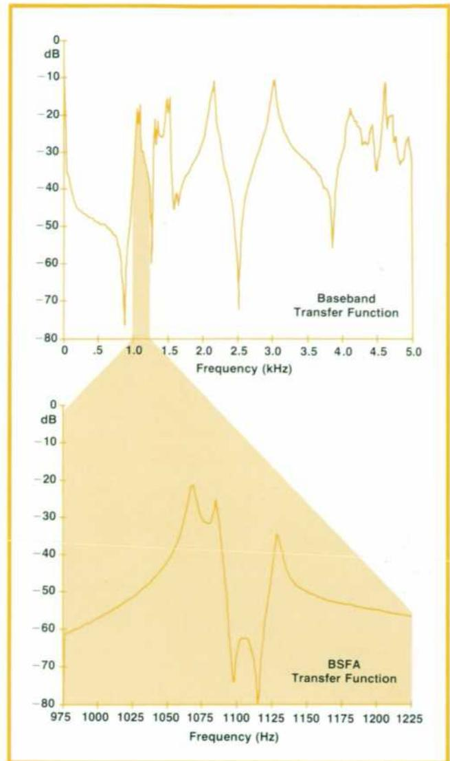
**Fig. 3.** In this mechanical impedance measurement on a squeaky automobile disc brake rotor, BSFA made possible an accurate determination of the modes of vibration and the damping associated with each mode.
