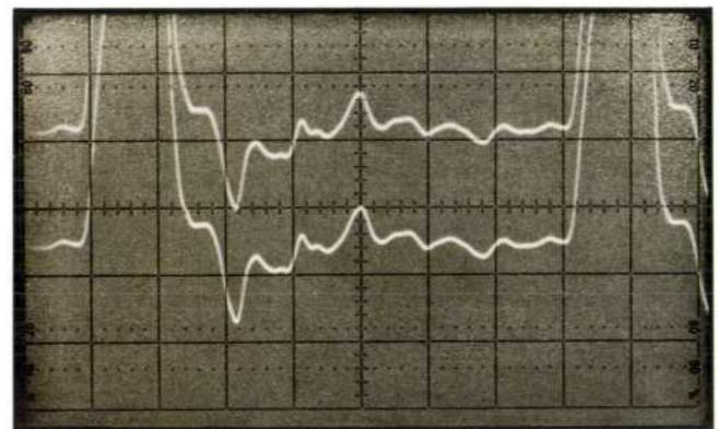
**Fig. 9.** Double-exposure photo shows how point-to-point voltage measurements are made. The reference point is first brought to a horizontal graticule line, in this case the center line (upper trace), with the vertical position control. The REF SET button is pressed, and the other point is brought to the same line (lower trace). The digital readout displays the voltage difference between the two points.
