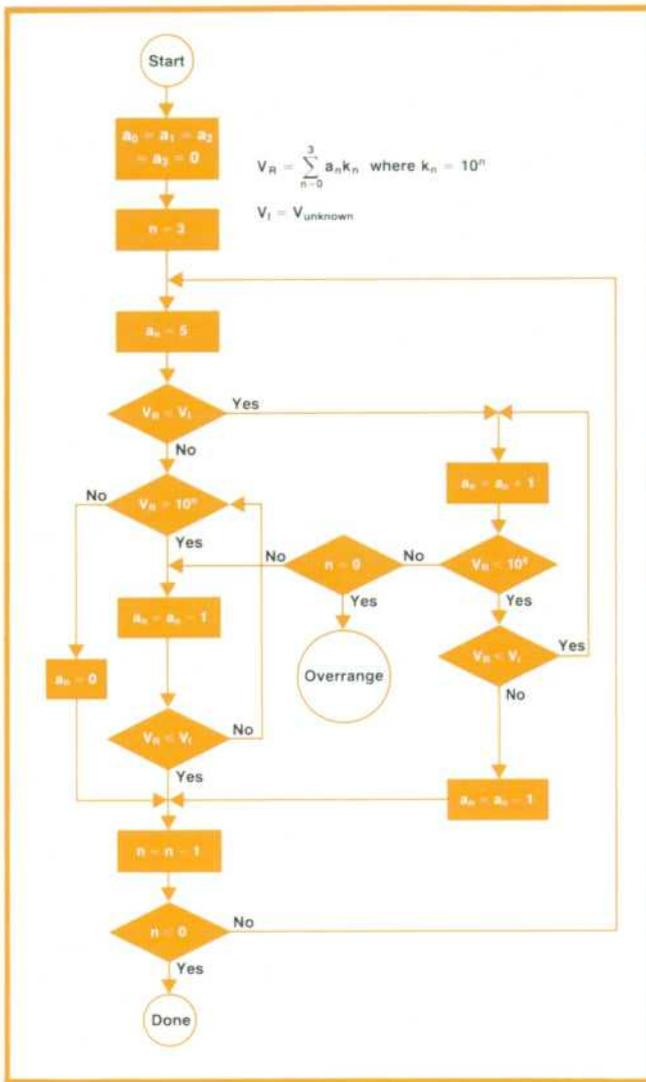
Fig. 11. Flow diagram of a voltage measurement.
