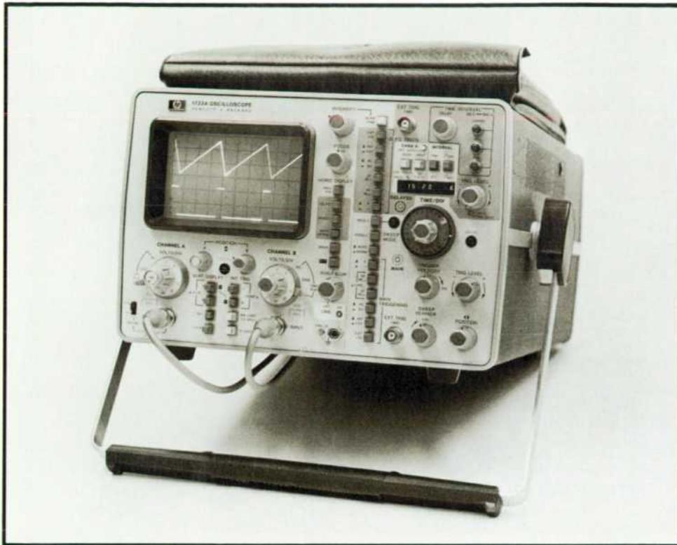
**Fig. 1.** Model 1722A Oscilloscope is a high-performance dual-channel instrument with 1.3 ns rise time, 50Ω or 1MΩ/11pF input impedance, sweep times to 1 ns/div, and the dual-delayed sweep that provides higher accuracy, resolution, and convenience in time-interval measurements. Its LED display gives direct readout of time intervals, frequency (1/TIME), and voltage.
