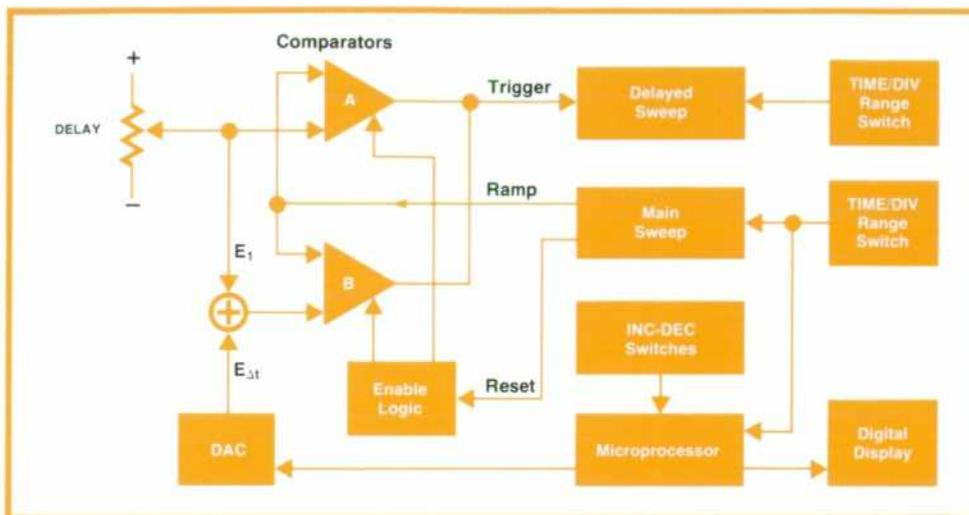
**Fig. 3.** The dual delayed sweep uses two comparators that are enabled alternately. Comparator A enables the main sweep ramp to trigger the delayed sweep when the ramp reaches the  $E_1$  level. On the next main sweep, comparator B enables the main sweep to trigger the delayed sweep at a later time when it reaches the  $E_1 + E_{\Delta t}$  level.
