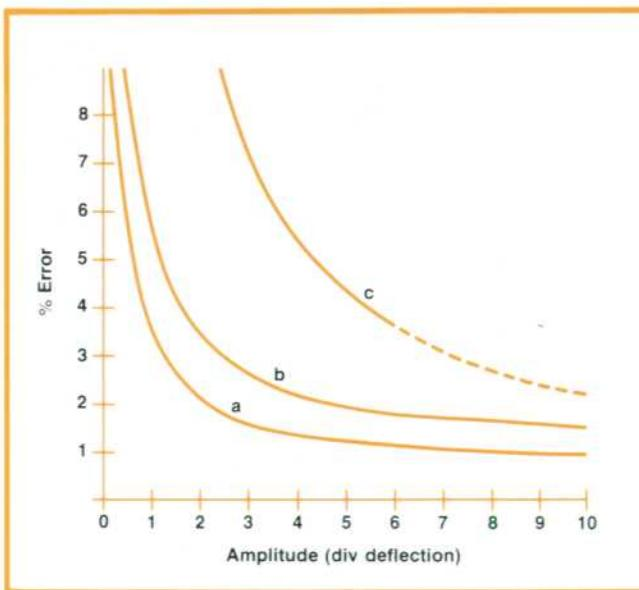
**Fig. 8.** Curves show specified accuracy of the Model 1722A Oscilloscope in voltage measurements (a and b) as compared to a conventional oscilloscope (c). Curve "a" is for dc voltage measurements. Curve "b" is for point-to-point measurements.
