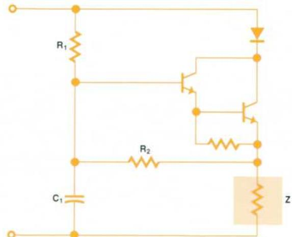
left connected without causing signal distortion. Two circuits connected in parallel opposition enable currents of either polarity to be accommodated.
