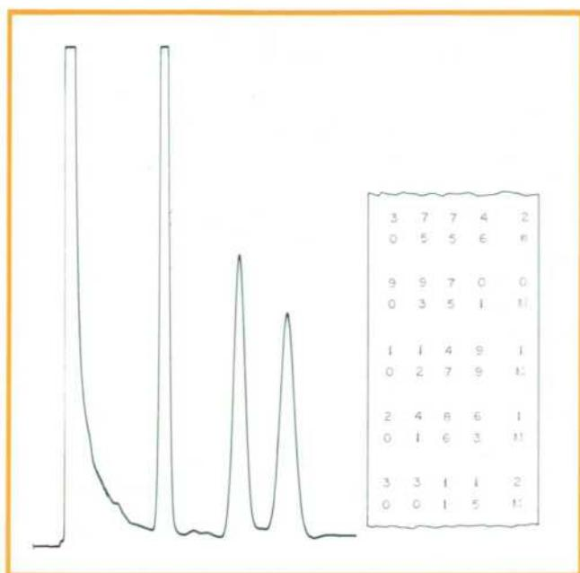
**Fig. 2.** Integrator printout with the corresponding chromatogram. The lower number of each pair gives the retention time in hundredths of minutes. The upper number gives the area count in  $\mu\text{V}$ -seconds with the digit in the right-hand column representing a power of 10 multiplier, e.g. 3311 2 means  $3311 \times 10^2$ .
