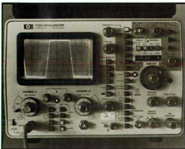
**Fig. 2.** Two markers are positioned to indicate the start and stop regions of a time-interval measurement and the digital readout shows the time interval between the markers. The example here shows the pulse width to be 18.80 μs.
