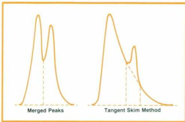
**Fig. 5.** Areas of merged peaks (left) are separated by a line dropped from the valley to the baseline. The area of a small peak riding on a tailing peak (right) is computed using the tangent line as a baseline. The area in the trapezoid below the tangent line is allocated to the tailing peak.
