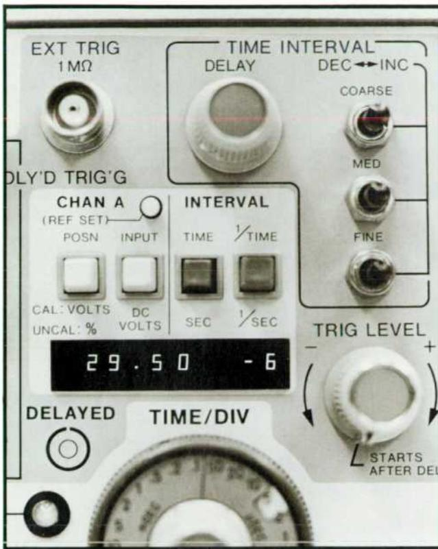
Fig. 5. The microprocessor is activated by pressing one of the function buttons (POSN, INPUT, TIME, 1/TIME). If any of the oscilloscope controls are not set appropriately for the measurement selected, the digital readout displays "0".
