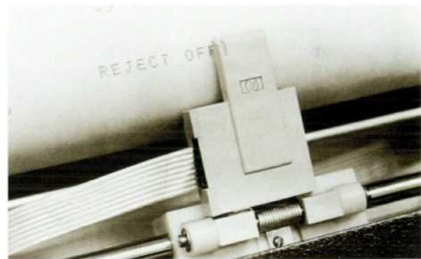
**Fig. B.** Thermal print-head mounts on the recorder's carriage.
