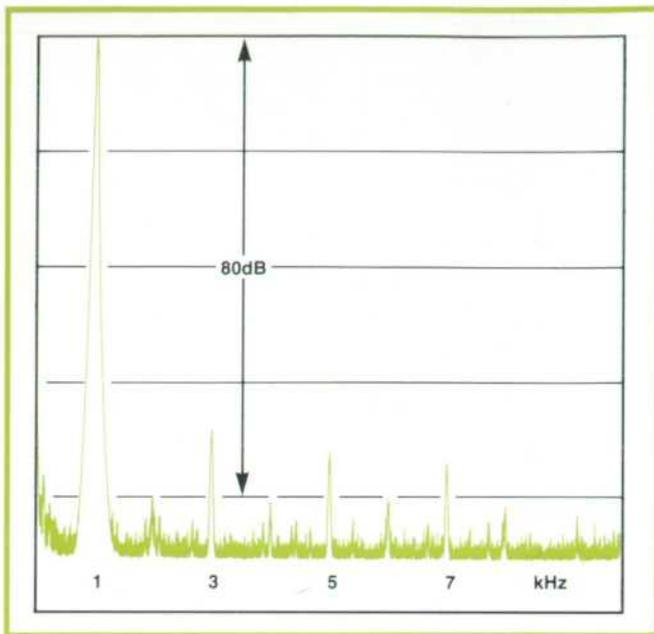
Fig. 6. Frequency spectrum of the synthesizer output (before modulation) when generating 1 kHz.
