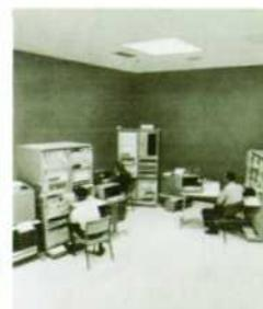
**Cover:** *In this distributed computer system, a 9700A Distributed System Central Station collects data from two satellite automatic test systems dedicated to measurement tasks. Test programs for the satellites are developed at the central station as a background activity. Communication is over hard-wired cable when the systems are as close as these or as much as two miles apart. Common-carrier facilities are used for more wide-spread networks.*
