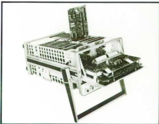
Fig. 10. Circuits are readily accessible for service.
