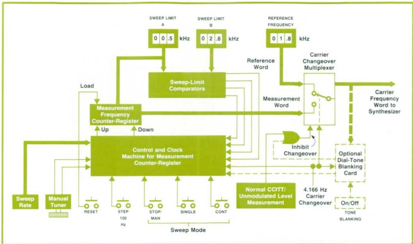
Fig. 7. Carrier frequency control logic generates a digital word corresponding to the synthesizer output frequency desired.
