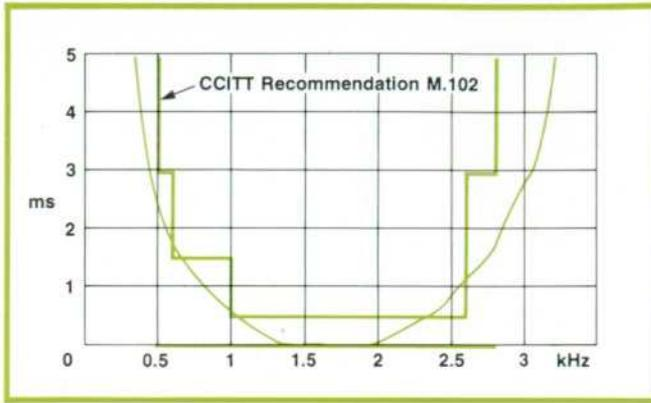
**Fig. 3.** Recording of a typical group delay measurement, this one being made over an international data circuit that included two satellite hops. The recording shows that the channel does not quite meet the requirements of CCITT performance recommendation M.102 and thus needs suitable equalization near the band edges.
