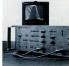
**Cover:** *The Model 8082A Pulse Generator's output for three different transition-time settings is shown on the sampling oscilloscope display in this triple-exposure photograph. The oscilloscope sweep time is 1 ns/div, demonstrating that transition*
