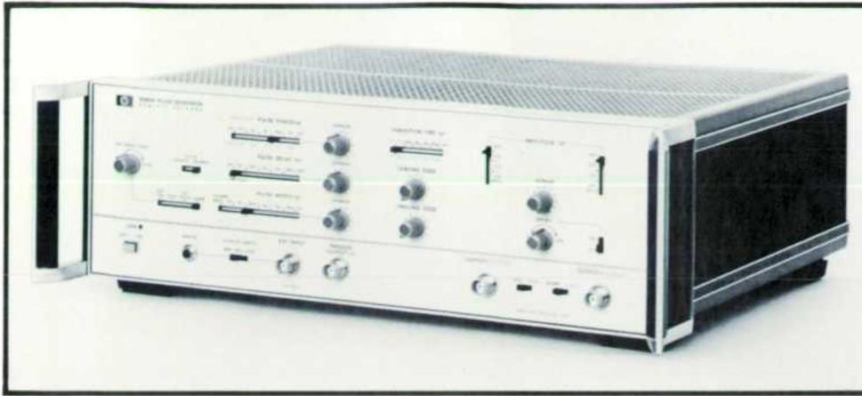
**Fig. 1.** Model 8082A Pulse Generator gives control of transition times over a range of 1 ns to 5 ms and pulse repetition rates as high as 250 MHz. Two outputs are provided, one the complement of the other. To speed operator familiarization, the slide switches concerned with time functions are arranged horizontally while those concerned with pulse amplitude are arranged vertically.
