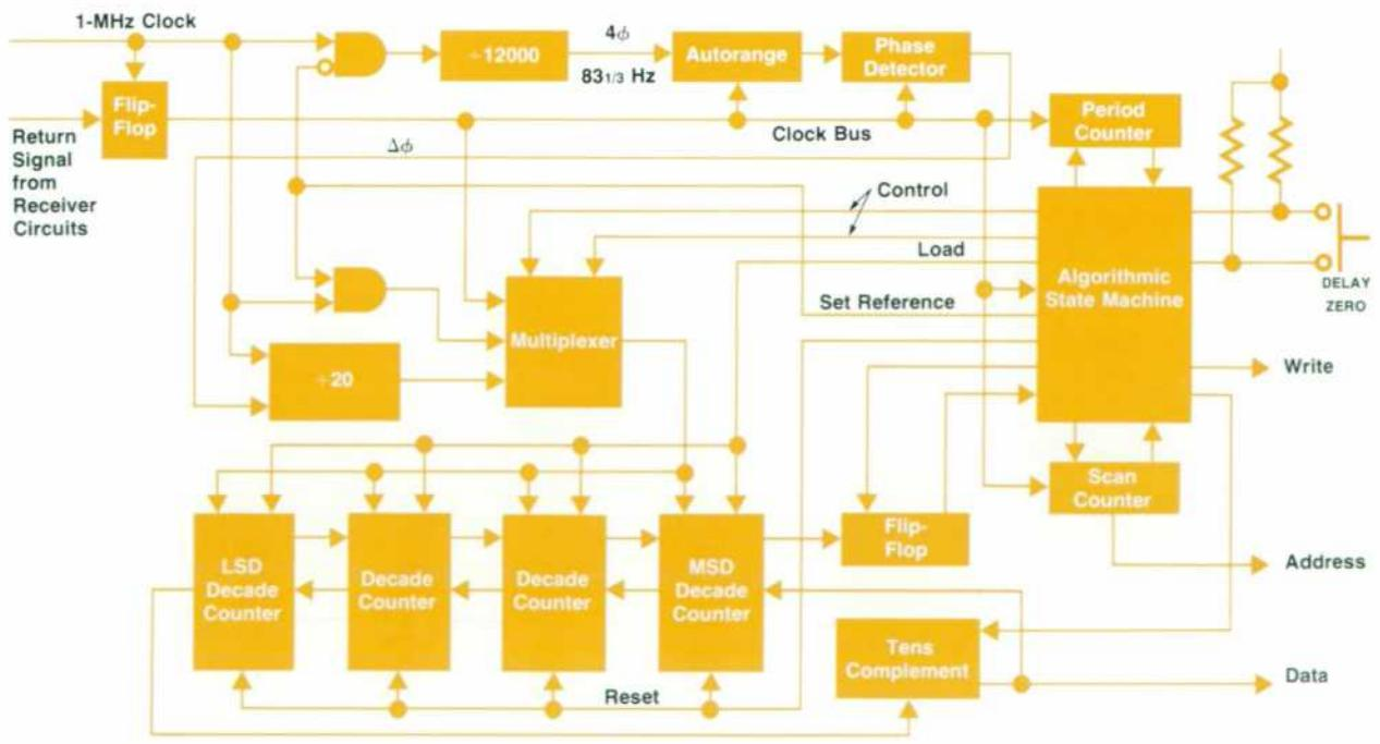
Fig. 3. 4940A envelope delay measurement circuits
