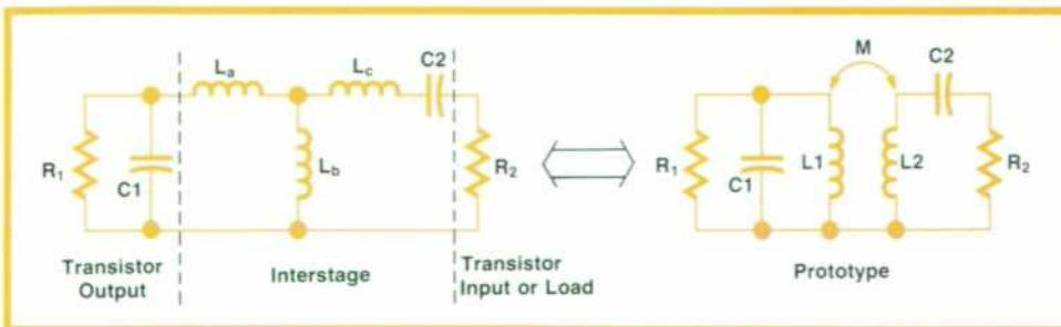
Fig. 4. Interstage coupling circuit at left was derived from the transformer-coupled prototype at right. Four-stage hybrid amplifiers using microwave chip transistors and this interstage achieve 30 dB of gain and 600-800 MHz bandwidth at 2.6 GHz.
