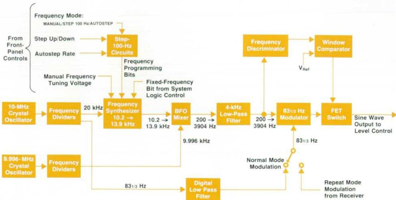
Fig. 1. 4940A sine wave transmitter block diagram
