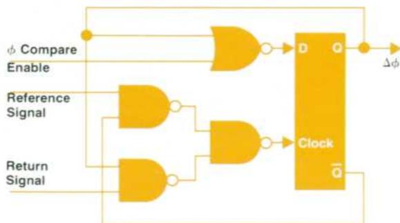
Fig. 4. Envelope delay phase detector
