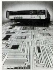
**Cover:** Model 4271A Digital LCR Meter is well suited for production measurements of chip capacitors and other components that are used on thin-film hybrid microcircuits like the one pictured here (it's actually a large photo of a microcircuit). Also easily measured by the new LCR Meter are varactor diodes, reed relays, delay lines, pulse transformers, and many other components, discrete and otherwise.
