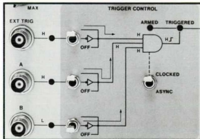
**Fig. 3.** Trigger event that determines the start of the display is defined by a combination of up to three HIGH or LOW logic states and a positive or negative-going edge. Here the Analyzer is set to trigger when there are logic HIGH's at the A and EXT TRIG inputs and a logic LOW at the B input, and the selected clock-pulse edge occurs.
