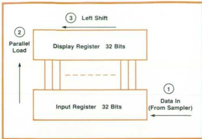
**Fig. 11.** Logic Analyzer displays data with oldest information at the left. At clock rates below 1 kHz the three steps shown occur on each clock cycle. The result is that each bit is displayed, properly positioned, as soon as it is entered. Data does not appear to shift in and is viewable while the display is being loaded.
