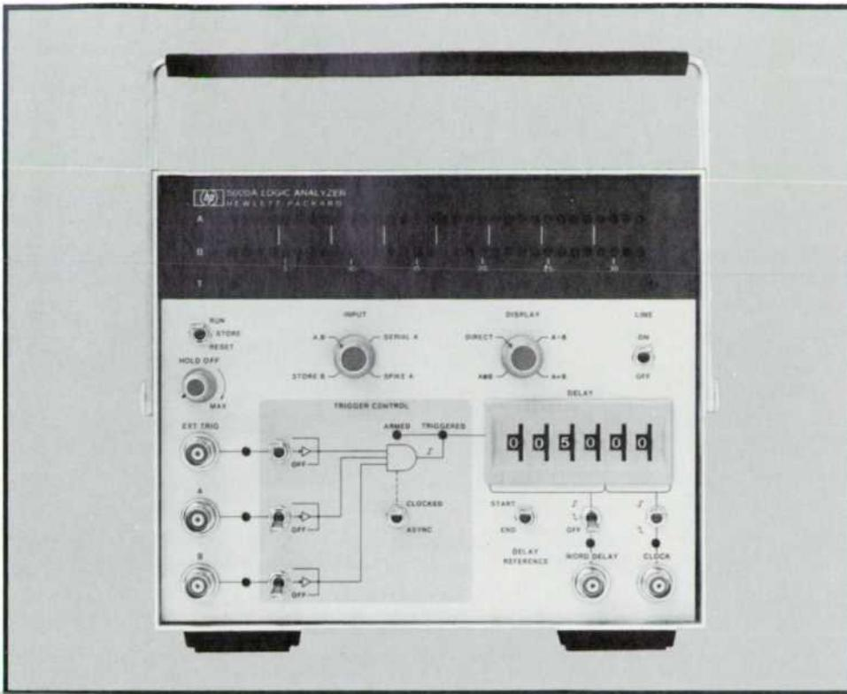
**Fig. 1.** Model 5000A Logic Analyzer's two rows of 32 light-emitting diodes display the sequences of logic states at the A and B inputs. Positive and negative delay, combinatorial triggering, storage, spike detection, and several display modes help solve a multitude of digital measurement problems in design and troubleshooting.
