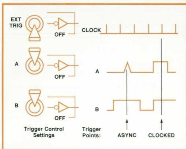
**Fig. 10.** In CLOCKED mode, the Logic Analyzer monitors its inputs for the trigger condition only at the selected clock edge. In ASYNC mode, triggering occurs as soon as the trigger condition appears at the inputs. Triggering is always edge-sensitive.
