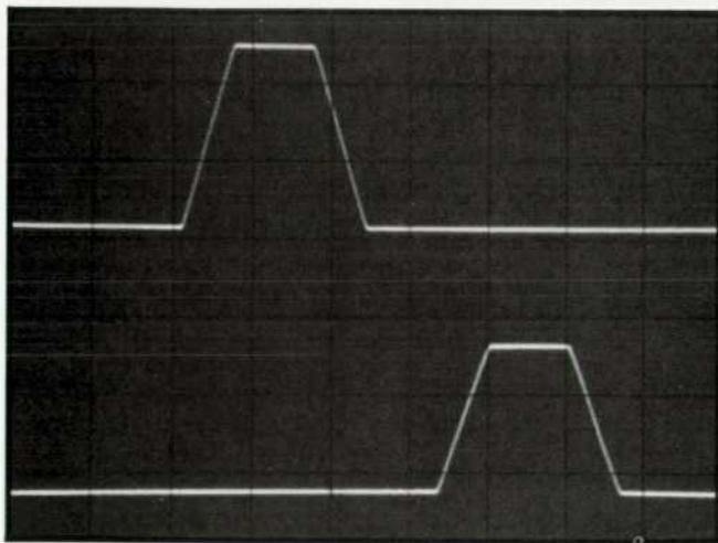
**Fig. 2.** Dual-trace oscilloscope shows how pulses in channel B can be delayed with respect to channel A, giving two-phase clock pulses.
