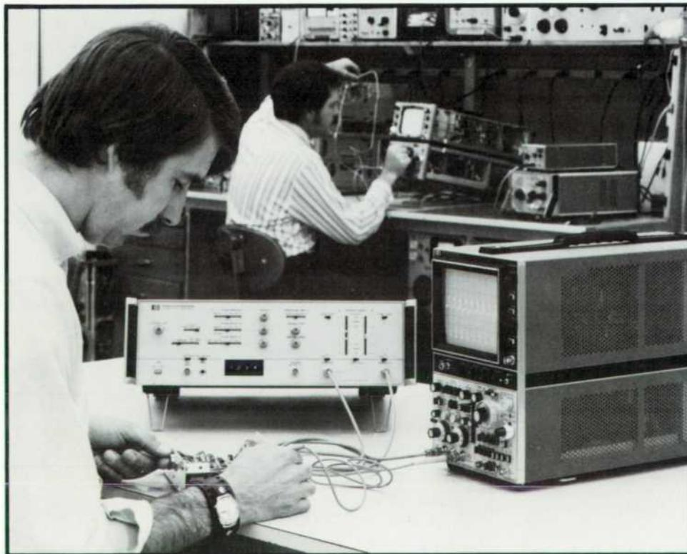
**Fig. 1.** New Model 8015A 50 MHz Pulse Generator has two outputs with individual control of amplitude, polarity, and baseline level for each. The arrangement of the controls simplifies operation. The instrument shown here is equipped with the optional burst mode of operation.
