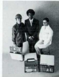
**Cover:** *A diversity of users calls for a diversity of calculating capabilities, and the 9800 Series has it. Models 10, 20, and 30 are three quite different calculators, but all offer the flexibility of plug-in read-only memories, internally expandable read/write memory, and numerous peripheral devices.*
