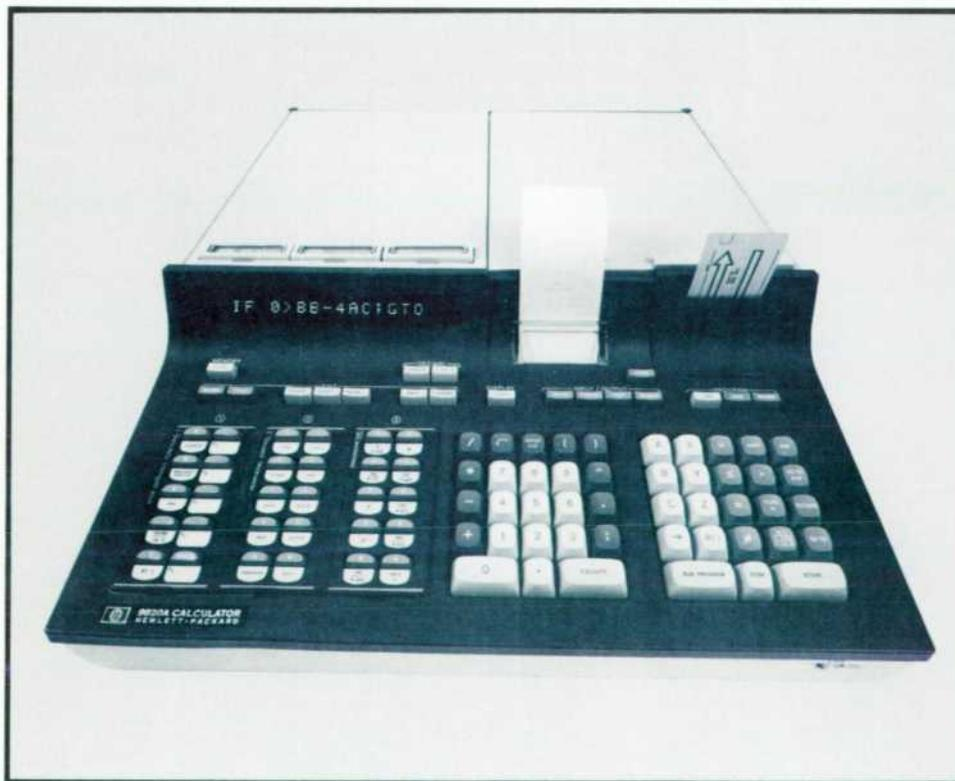
**Fig. 1.** Model 20 of the 9800 Series has a 16-character alphanumeric LED display that shows several keystrokes or program steps in context. Special features are a natural algebraic language, an interactive mode of operation, and plug-in modules that define the functions of the three lefthand keyblocks.
