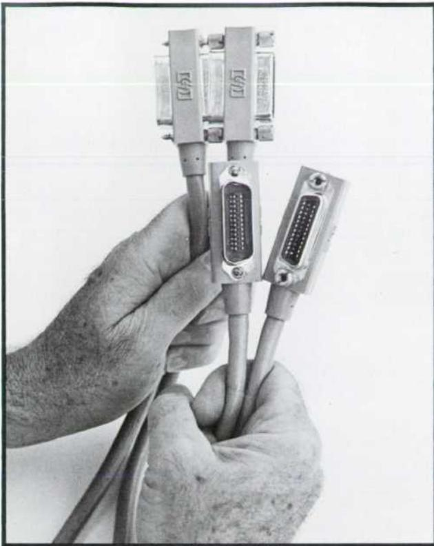
**Fig. 1.** Interconnecting cables used with interface system have dual connectors. These can be stacked to accommodate variety of physical layouts by allowing more than one cable to be attached to any device.
