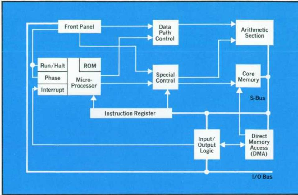
**Fig. 1.** Block diagram of Model 2100A Computer. The micro-processor is a computer within a computer, running micro-programs stored in its read-only memory (ROM). There's a microprogram for each user instruction.
