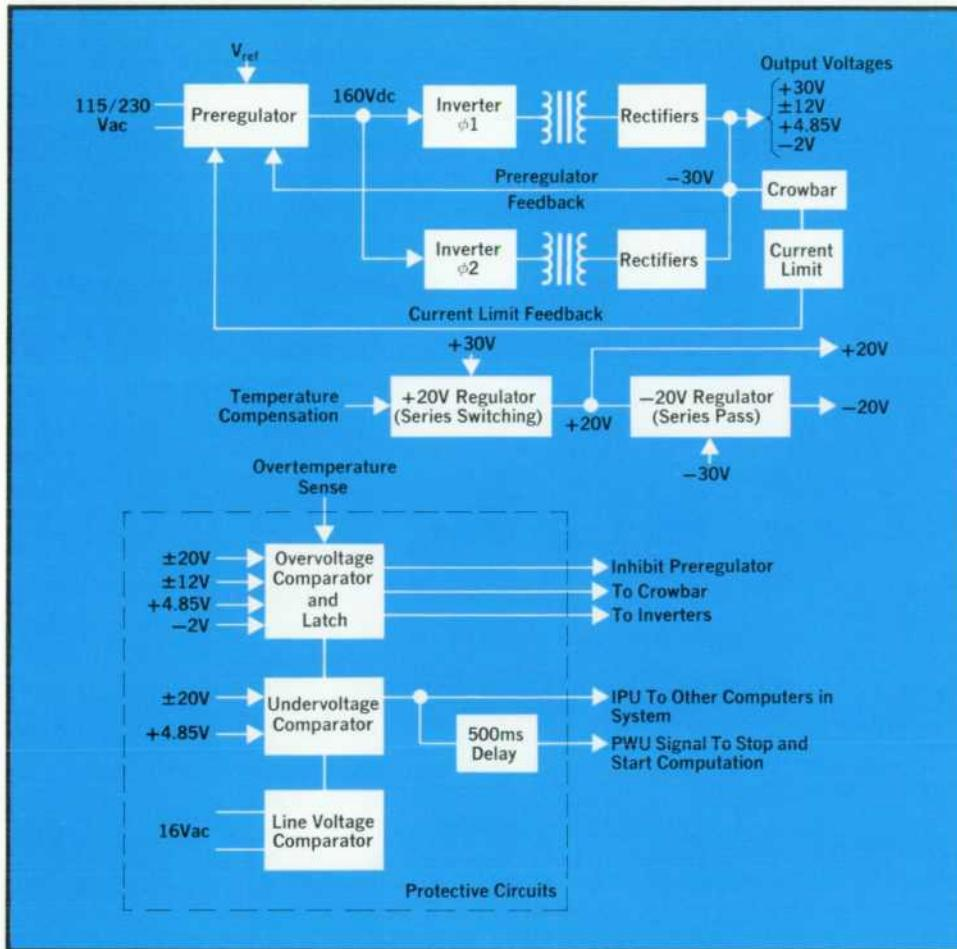
Fig. 1. Power supply for 2100A Computer provides 500 watts at seven regulated output voltages, yet occupies only 800 in<sup>3</sup>. Computer, software, and supply are fully protected.
