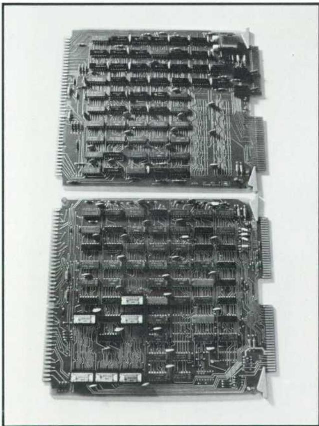
**Fig. 2.** Basic 2100A ROM consists of six packages, each containing one 1024-bit bipolar integrated-circuit chip. (On this prototype board the ROM packages are mounted in sockets.) Empty spaces on the boards can be loaded with three more six-package ROM groups to extend the instruction set. A six-package floating-point option is now available.
