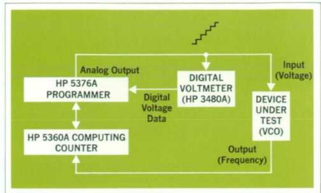
Fig. 7. Computing-counter system to measure integral nonlinearity.
