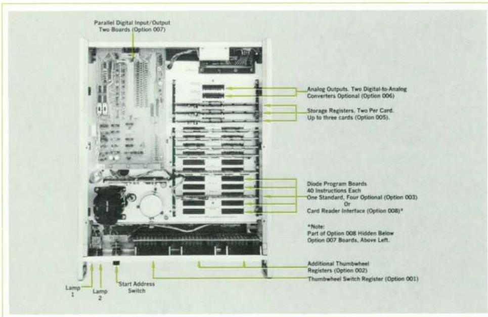
**Fig. 2.** Most programmer capabilities come as plug-in options, requiring only a screwdriver to install. Systems can be tailored to fit the requirements of a given application, and still be readily modified later.
