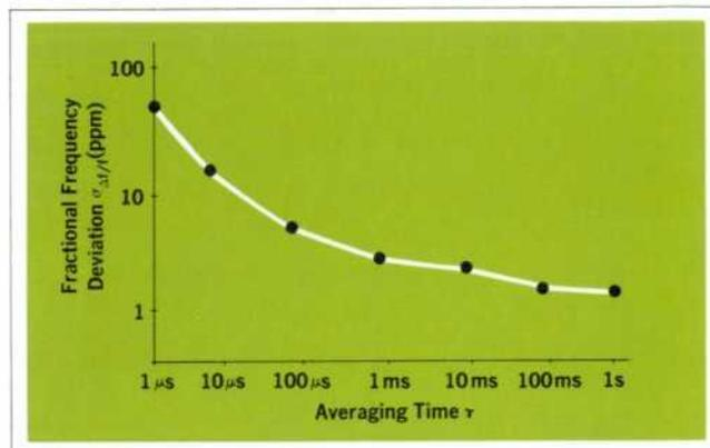
Fig. 4. Short-term stability of an oscillator. The computing-counter system can be programmed to make the frequency measurements and perform the computations needed to obtain a direct readout of  $\sigma_{\Delta f/f}$ .
