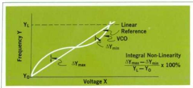
Fig. 6. Integral nonlinearity of a voltage-controlled oscillator.
