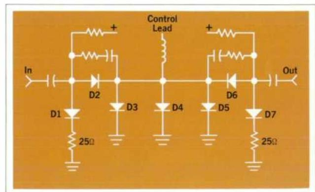
Fig. 16. Equivalent circuit of PIN diode modulator-attenuator.
