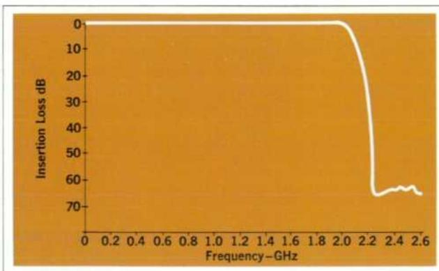
Fig. 15. Frequency response of typical 2-GHz low-pass filter.
