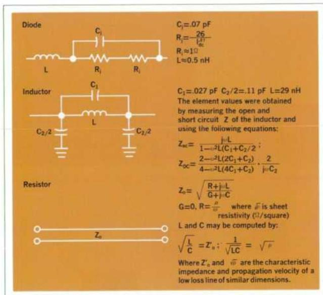
Fig. 17. Equivalent circuit elements of PIN modulator-attenuator.
