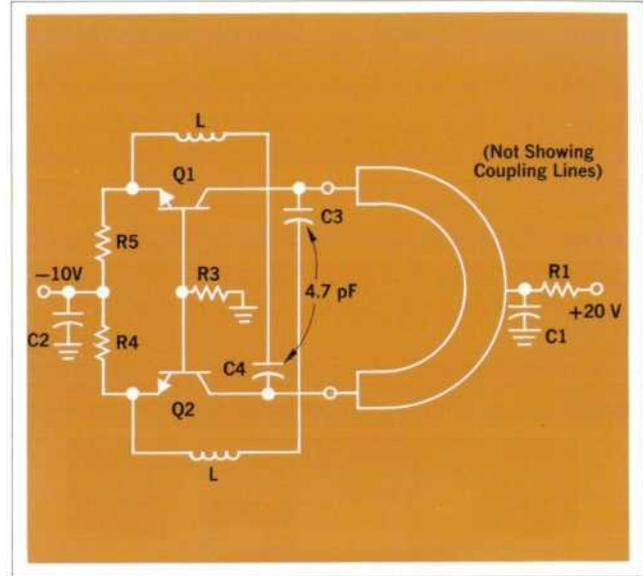
Fig. 9. Simplified schematic diagram of 4.3 GHz oscillator.
