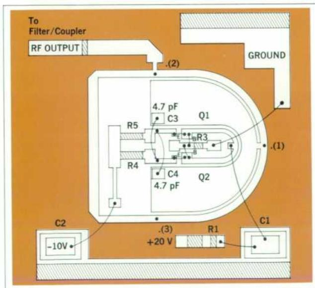
Fig. 12. Layout of 4.3 GHz push-pull microcircuit oscillator.
