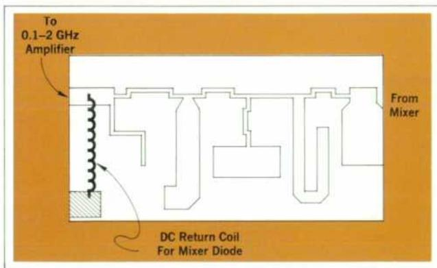
Fig. 14. Layout of 2-GHz low pass filter microcircuit.
