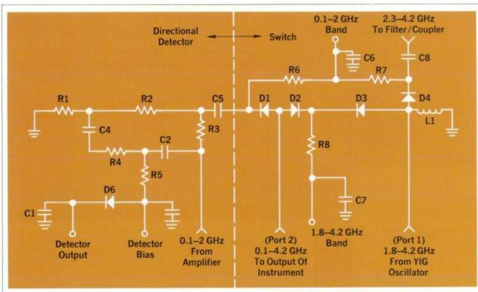
Fig. 2. Schematic diagram of directional detector/switch microcircuit.
