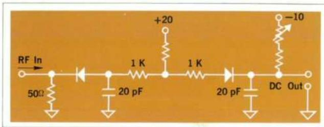
Fig. 19. Temperature-compensated crystal detector.
