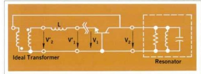
Fig. 10. Equivalent circuit of 4.3 GHz oscillator.
