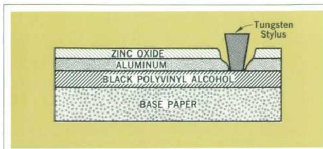
Fig. 3. HP electrosensitive paper is layered as shown here. The tungsten stylus burns through to the black layer.
