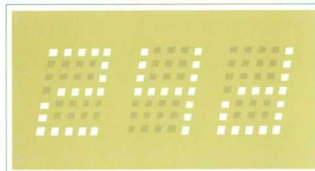
Fig. 6. How the 5 by 7 dot characters are generated.
