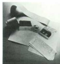
*Cover: Marked cards, lower right, are used to enter programs and data in the Model 9100 Calculator System through the Model 9160A Card Reader, center. Hard copy output, upper left, is produced by the Model 9120A Printer, mounted on the calculator. The HP Model 9101A Extended Memory, left, greatly increases the computing power of the system.*
