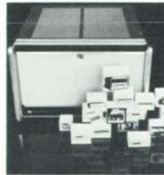
*Cover: Represented here by photo blocks are some of the digital devices that can communicate with each other by means of Model 2570A Coupler/Controller. Computers, calculators, stimulus and measuring instruments, data recording and data entry devices, acoustic couplers for time-shared systems, and many others can be building blocks for a variety of systems built around the coupler/controller.*
