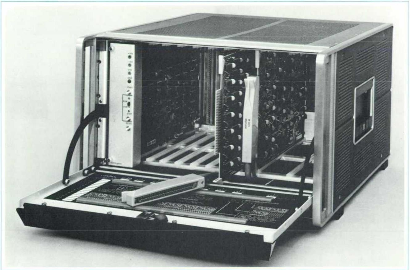
**Fig. 1.** Model 2570A Coupler/Controller is a programmable two-way data link by which as many as eight digital devices can communicate with each other for purposes of control and data transfer. It can serve as the nucleus of a large number of measurement, control, and data acquisition systems. Plug-in I/O cards connected to instruments, peripherals, and computing machines translate various codes to ASCII. Information is exchanged between cards in ASCII code via a bus in the backplane.
