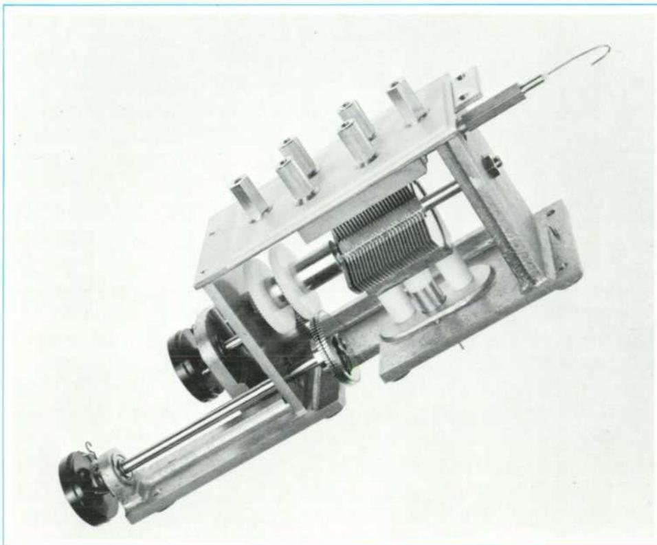
**Fig. 5.** This precision tuning capacitor is the reactance standard in the instrument.
