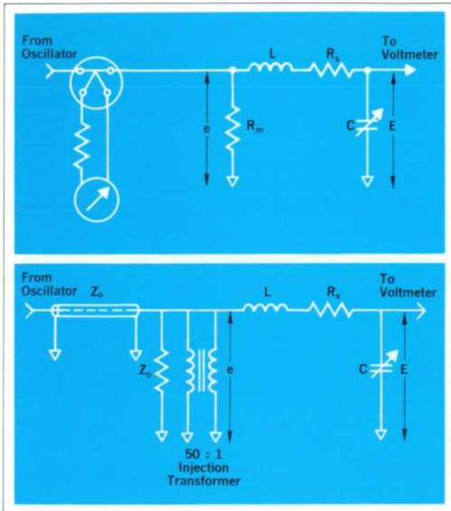
**Fig. 4.** Constant current injection system (a) used in the older Model 260A Q meter uses a thermocouple that can be easily damaged. Constant voltage injection system (b) used in the new Model 4342A Q Meter uses a transformer with an output impedance of only 1 milliohm.
