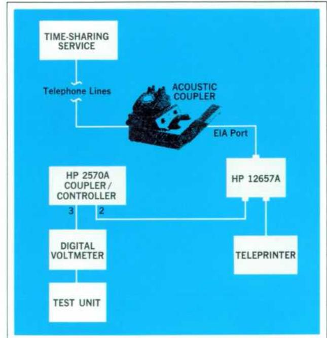
**Fig. 1.** Model 2570A Coupler/Controller acts as a data link between instruments and time-shared computers, so even a simple system can have the benefits of computer control and data processing at the relatively low cost of a time-sharing terminal. In this example, the average of several digital voltmeter readings is computed and printed out.
