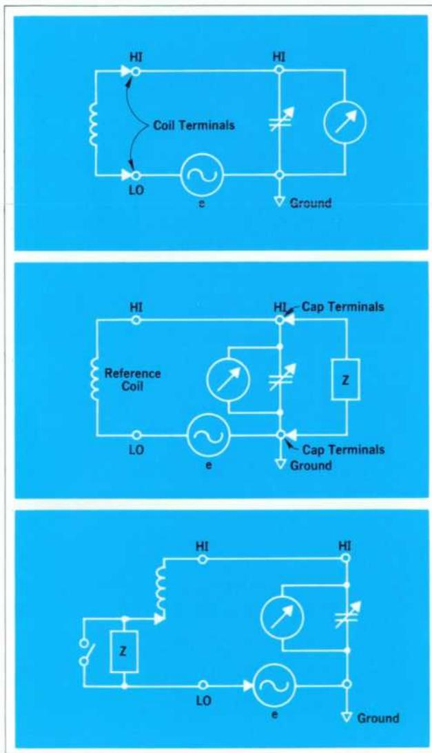
Fig. 7. Three ways in which components are measured with the Q meter. Most components in the medium inductance range ( $0.09 \mu\text{H}$  to  $1.2 \text{ H}$ ) are connected directly (a). High impedance components are connected in parallel (b) with the capacitor, and low impedance components use the series connection (c).
