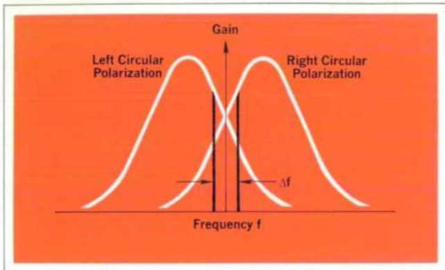
**Fig. 3.** Two frequencies are derived from the single-mode laser by Zeeman splitting. An axial magnetic field causes the single line to split into two lines. The two frequencies have opposite circular polarizations.
