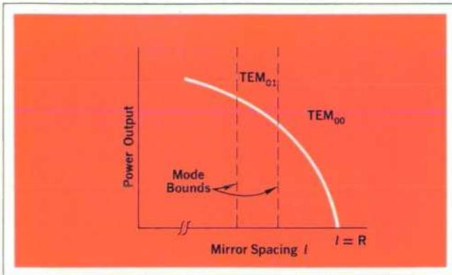
**Fig. 1.** Laser power output versus mirror spacing for a given diffraction aperture (bore diameter), showing typical transverse-mode bounds. New HP laser operates in  $TEM_{00}$  mode only, but as close to  $TEM_{01}$  region as possible, so as to maximize power output.
