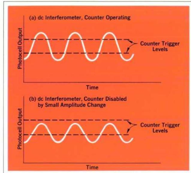
**Fig. 5.** Most laser interferometers use dc systems in which intensity changes due to aging or air turbulence can interfere with triggering and cause improper counting. The new HP interferometer uses an ac system which doesn't have this problem.
