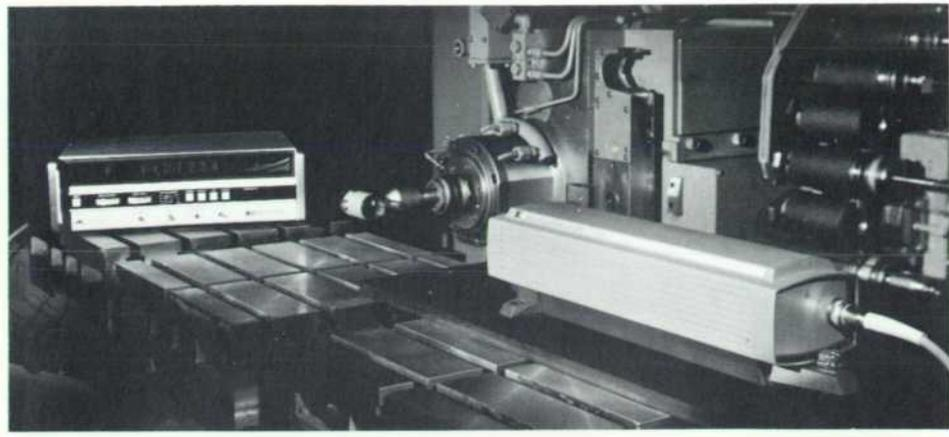
**Fig. 1.** Model 5525A Laser Interferometer is a rugged, easy-to-use distance-measuring system with a range of 200 feet, accuracy better than 5 parts in 10<sup>7</sup>, and usable resolution better than one microinch. Its new two-frequency laser warms up instantly, runs cool, and doesn't mind air turbulence, the most common cause of poor interferometer performance.
