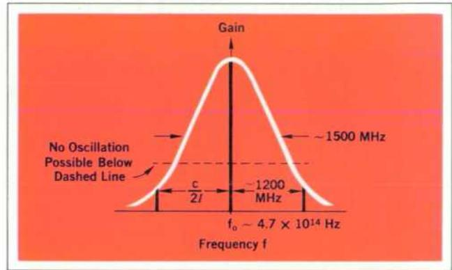
**Fig. 2.** This is the Doppler-broadened gain curve for the 6328A (632.8 nm) line of helium-neon. In the new HP laser, cavity length ( $l$ ) is about 13 cm, so only a single longitudinal mode can oscillate.
