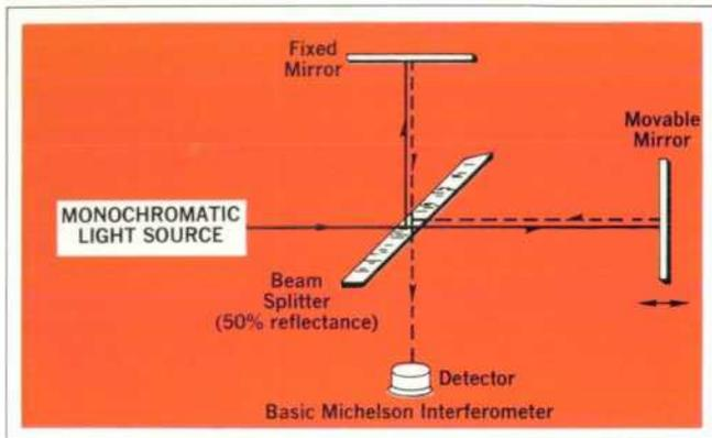
**Fig. 4.** Laser interferometers are based on the Michelson interferometer of the 1890's. If one of the two mirrors moves, the observer sees the light repeatedly increasing and decreasing in intensity as light from the two paths alternately adds and cancels. Each cycle of intensity corresponds to a half-wavelength of mirror travel. If the wavelength of the light is known, intensity cycles can be counted and converted to distance traveled.
