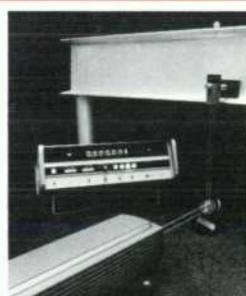
**Cover:** Model 5525A Laser Interferometer has one-microinch resolution (0.4 microinch when displaying in metric units), but what does this mean? We decided to find out, and this cover is the result. That's a four-foot-long aluminum beam, and the penny deflects the center of it about a microinch.
