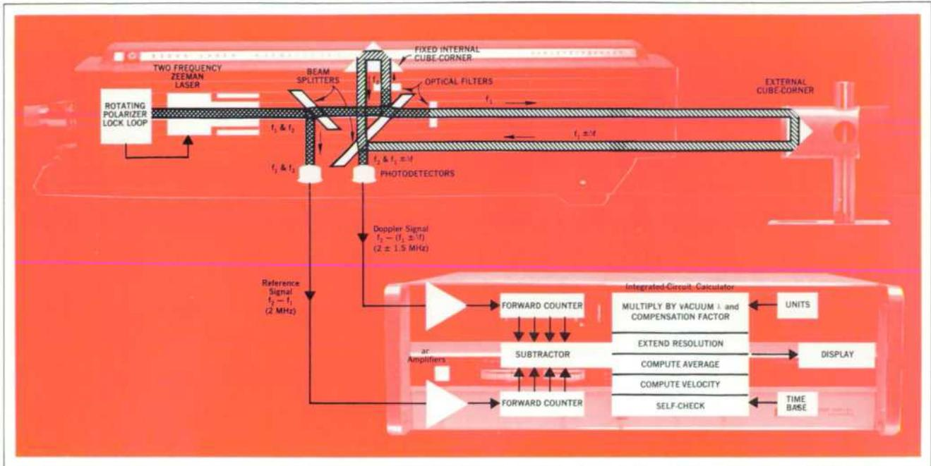
**Fig. 6.** In the HP interferometer, two frequencies are generated by the laser and separated by optical filters of opposite circular polarizations. The beam of frequency  $f_1$  is Doppler-shifted as it bounces off the moving reflector. The returned beam is optically mixed with the beam of frequency  $f_2$  and the difference frequency is detected, amplified, counted, and converted to distance traveled.
