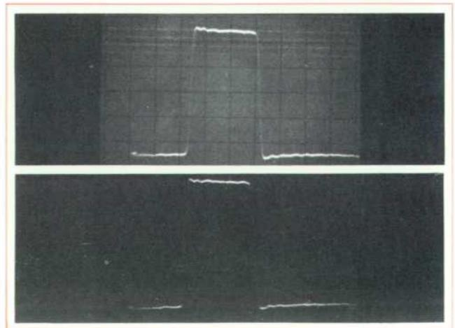
**Fig. 2.** Trace writing speed is increased by film and phosphor 'fogginess' (upper trace) over speed obtained without fogginess (lower trace), as shown by leading and trailing edges of fast pulse ( $t_r = 1.5$  ns). Internal flood gun in Model 183A Oscilloscope fogs film and phosphor automatically in synchronism with horizontal sweep.
