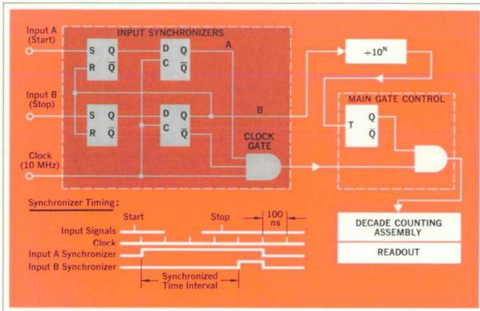
**Fig. 7.** Synchronizing circuit makes certain that a multiple-time-interval average will tend towards the true value. In measuring 205 ns, for example, the counter will accumulate two counts 95% of the time and three counts 5% of the time, provided the repetition rate of the unknown intervals isn't synchronous with the 10 MHz clock.
