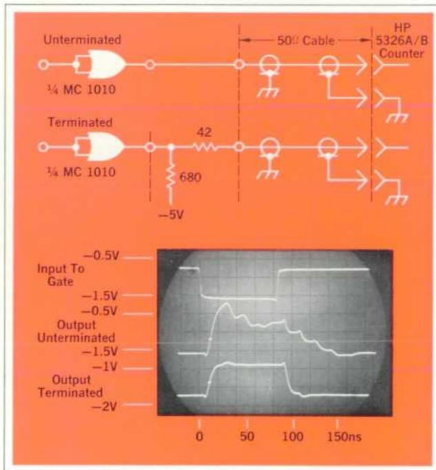
**Fig. 3.** Output of an ECL gate connected to Model 5326A Timer/Counter, first using only a 50Ω cable (middle trace) and then a 50Ω cable with the proper series termination. Reflections resulting from improper termination can cause double counts, incorrect readings.
