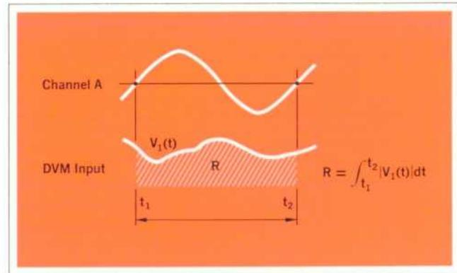
**Fig. 9.** By remotely programming Model 5326B for both PERIOD A and DVM, the instrument can be made to measure the integral of the DVM input over the period of input signal A. This is useful in scaling or units conversion. See Fig. 10.
