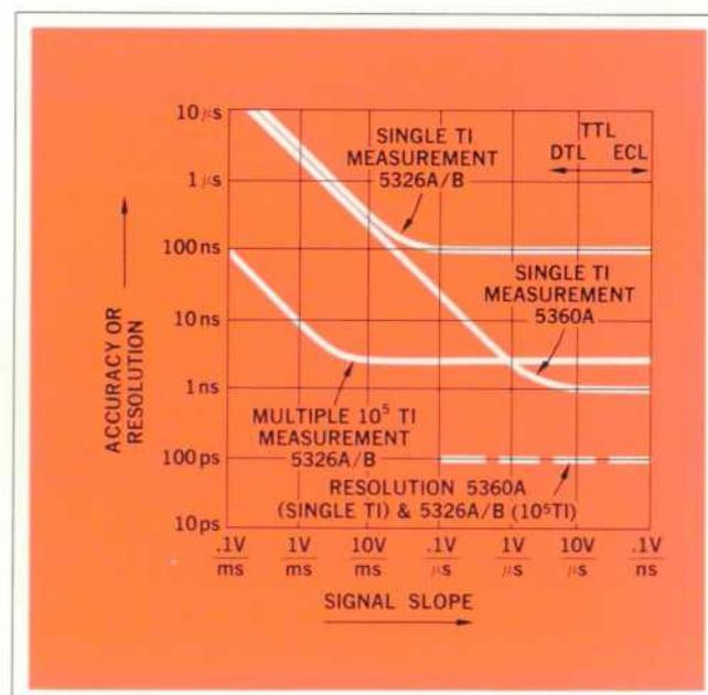
Fig. 1. In single time-interval measurements, Model 5326A/B Timer/Counter's accuracy is  $\pm 100$  ns and resolution is 100 ns. In an average of  $10^5$  measurements, accuracy is  $\pm 2$  ns, and resolution is better than 100 ps. Accuracy can be improved by calibration (see text). Model 5360A Computing Counter's accuracy and resolution are shown for comparison. Sloping parts of all curves are due to internal noise.
