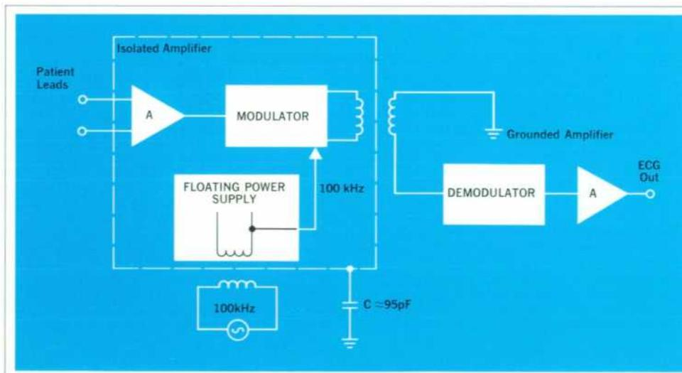
Fig. 5. AC coupling to isolated amplifier eliminates any dc connection between input and output. Input signal modulates 100 kHz carrier for coupling to external circuits. Demodulator recovers original input waveform. Supplying circuit power from 100 kHz oscillator rather than 60 Hz power line reduces need for tight coupling between power transformer windings.
