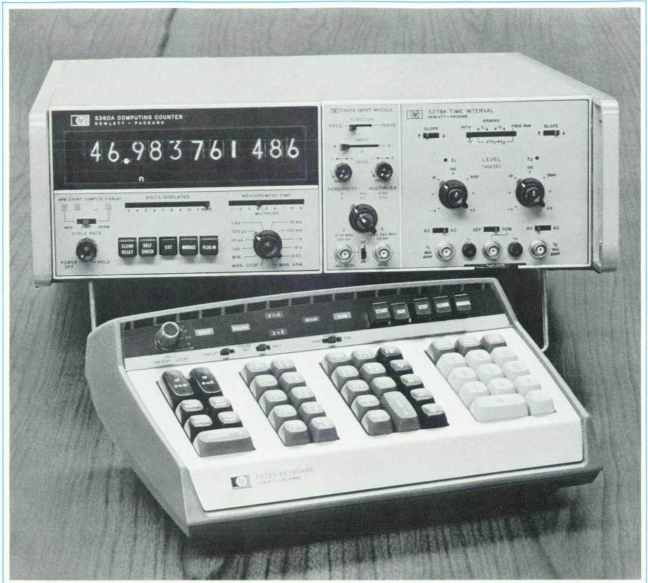
A Programmable Measurement/Computing System: Model 5360A Computing Counter with Model 5379A Time Interval Plug-in and the new Model 5375 A Keyboard
