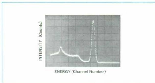
**Fig. 1.** Gamma-ray spectrum of  $Cs^{137}$  as seen by a scintillation detector is typical of multichannel-analyzer results. The information of interest—the energy and intensity of each peak—can't be read directly; it has to be extracted by computation.
