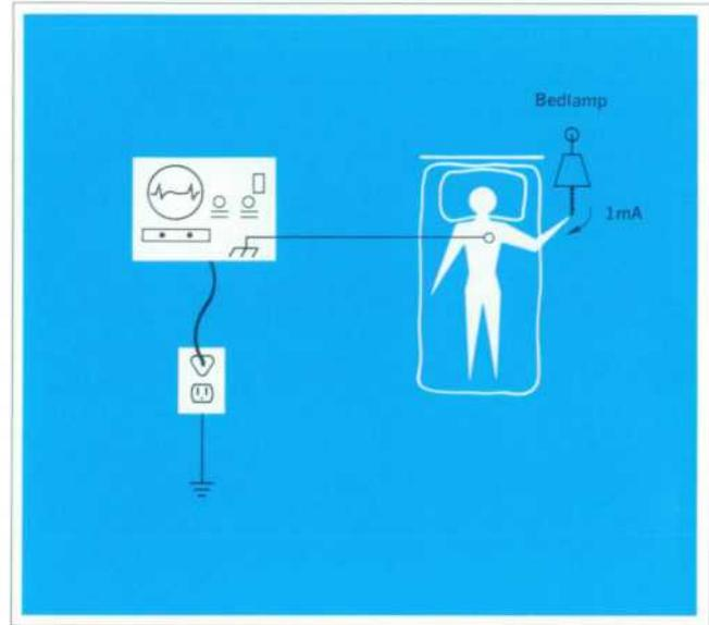
**Fig. 1.** Normally harmless leakage current in lamp can become dangerous if patient has internally attached electrodes.
