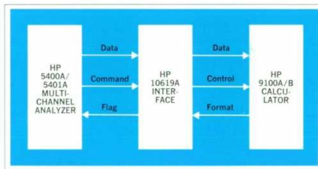
**Fig. 2.** Two interface cards plugged into the multichannel analyzer allow it to communicate with the HP calculator. The calculator is programmable, easy to use, and fast, and it can reduce most analyzer data just as well as a computer.
