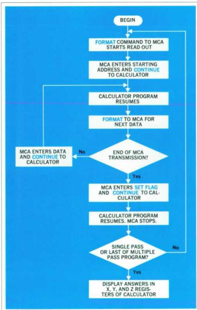
Fig. 3. Simplified flow chart of multichannel-analyzer/calculator operation.
