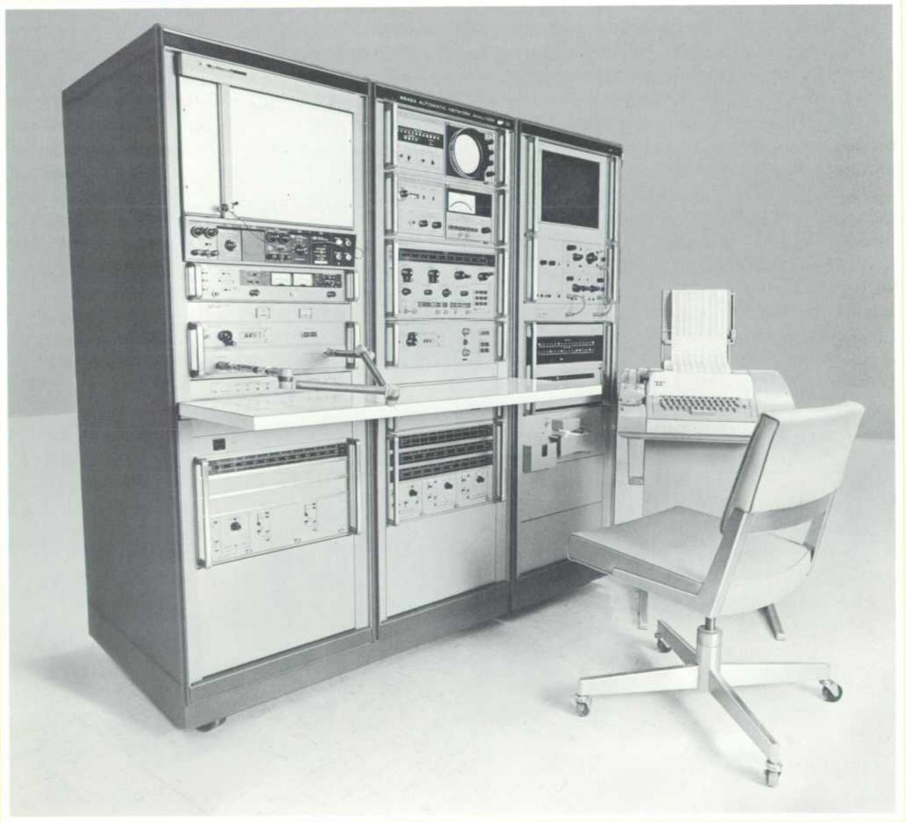
*Fig. 1. The automatic network analyzer system in this photo has an unusual number of readouts—note X-Y recorder, oscilloscope displays, and teleprinter. The number of possible configurations is almost unlimited.*
