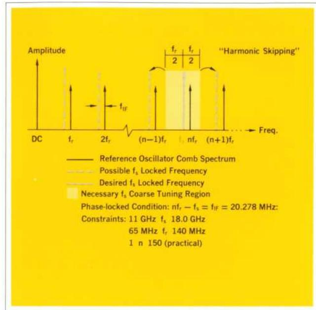
Fig. 6. Source phase-locks when  $nf_r - f_s = f_{IF}$ .
