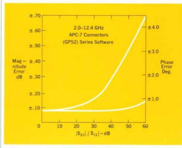
Fig. 2. Curves show complete accuracy results for HP Model 8743A Reflection/Transmission Test Set in the range 2.0 to 12.4 GHz. Dotted curve of Fig. 2b shows improvement in accuracy obtained when noise is reduced by a factor of 10.
