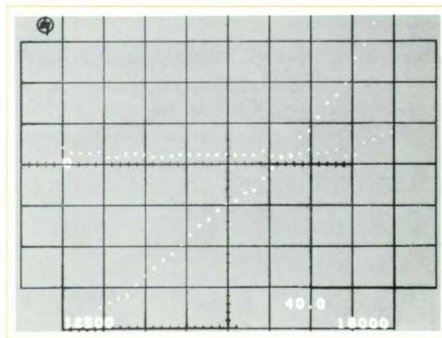
**Fig. 1.** Scope shows real and imaginary components of tuning cavity impedance. Resonant frequency is easily determined, as is value of impedance at resonance. Vertical scale +40 to -40  $\Omega$ , horizontal scale 12.5 to 18.0 GHz with one dot for each 150 MHz.
