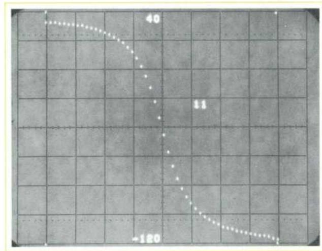
**Fig. 4.** Transmission and reflection characteristics of sharp filter (HP Model 536A Frequency Meter). Curve of transmission magnitude (above, left) is centered on 3 GHz, vertical scale 0.4 dB/division. Transmission phase characteristic (above, right) is shown at 2°/div. Magnitude (lower left) and phase (lower right) of reflection coefficients are shown. Scale factor for magnitude is 0.025/div, and for phase 20°/div.
