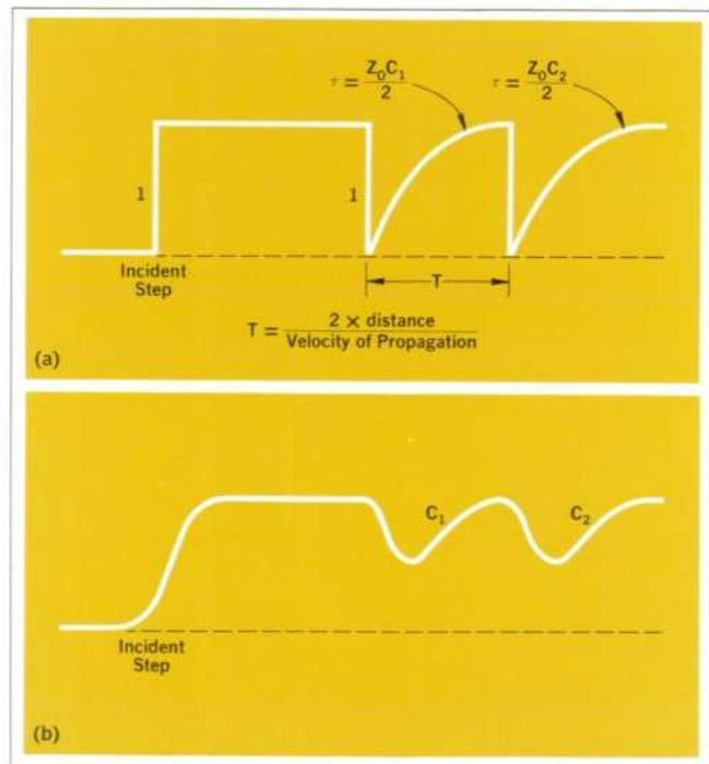
**Fig. 1a.** Response of ideal zero-risetime time-domain reflectometer to two capacitors bridging lossless line. Response of realizable (risetime-limited) time-domain reflectometer is shown in 1b.
