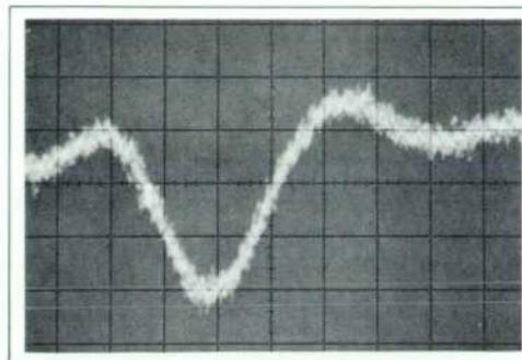
Fig. 4. Resolution obtainable with 1815A TDR system using 28ps sampling head and 20ps step generator. Reflection shown is from 0.02pF ( $2 \times 10^{-14}$  F) capacitor shunting 50  $\Omega$  transmission line. Vertical deflection factor: 0.005  $\mu$ /div; horizontal: 0.02 ft/div.
