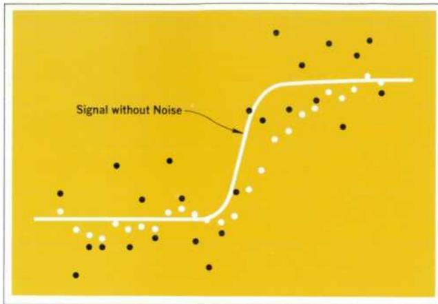
**Fig. 11.** Display of voltage step by sampling scope set for 100% sampling efficiency (black dots) and for 25% sampling efficiency (white dots). Note smoothing of response with reduced sampling efficiency, and consequent loss of risetime. (Horizontal dot spacing is exaggerated for purposes of illustration.)
