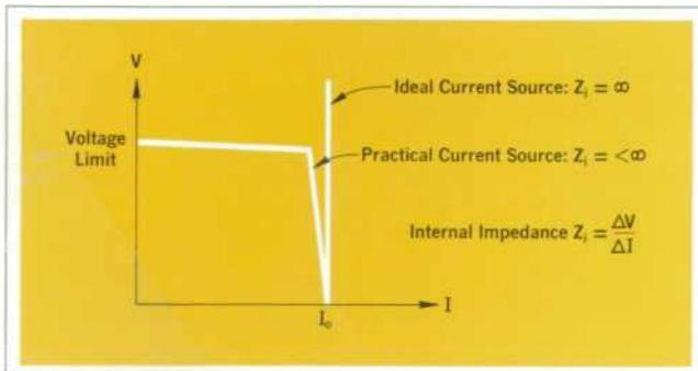
**Fig. 1.** An ideal current source has infinite internal impedance, delivers the same current,  $I_o$ , to any load, and supplies infinite voltage to an open circuit. A practical current source has a  $Z_i$  which is finite, but as high as possible. It should also have an adjustable voltage limit to keep the load from being damaged.
