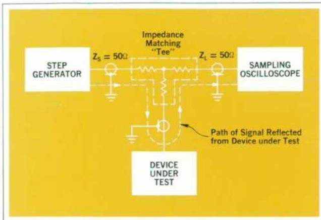
Fig. 2. Time domain reflectometer using ordinary lab instruments.
