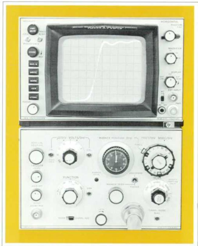
**Fig. 6.** Front panel view of Model 1815A TDR/Sampler plug-in in Model 181A Oscilloscope mainframe. Outer concentric control (FEET-NSEC/DIV) switches in decade steps so only decimal point placement need be considered in reading MARKER POSITION dial. Sweep magnifier (EXPAND) is on inner concentric knob and reads horizontal scale calibration directly.
