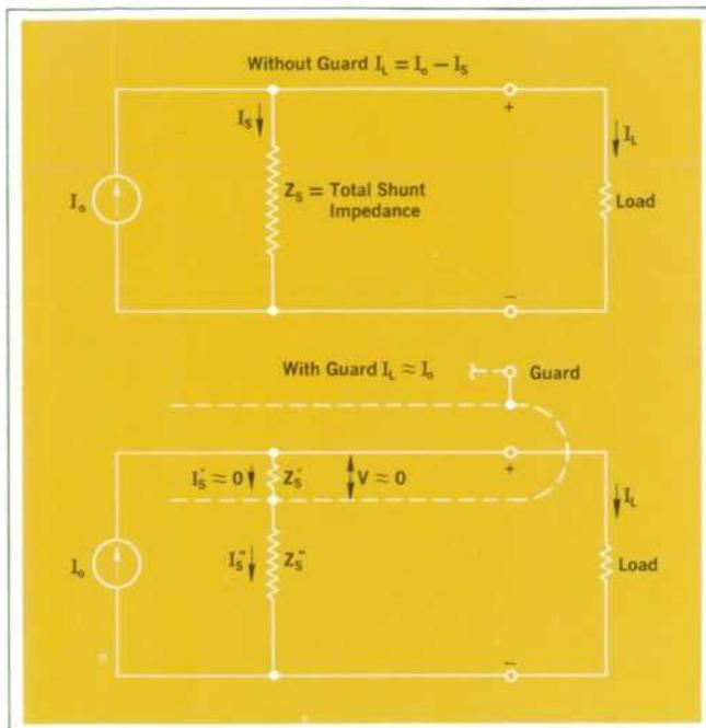
**Fig. 5.** The guard surrounding the positive output terminal splits the impedances through which leakage currents ( $I_s$ ) flow. The guard and the positive output terminal are kept at the same voltage, thereby keeping the leakage currents from degrading the regulation. The output voltage can be measured at the guard so the meter impedance doesn't shunt the load.
