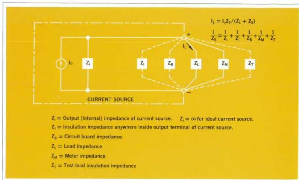
**Fig. 2.** The current regulation of a current source can be degraded by any impedance that shunts the load. If  $Z_1$  is high, meter and leakage impedances can be significant.
