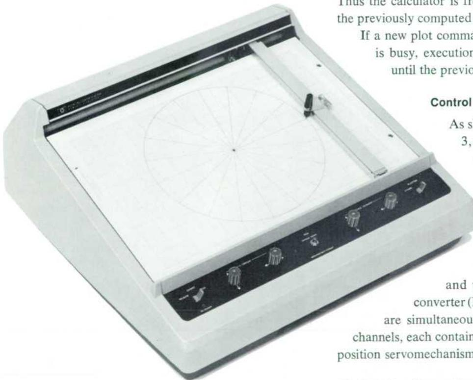
**Fig. 1.** This Model 9125A X-Y Plotter automatically plots solutions to problems solved by the HP Model 9100A Computing Calculator. Manual operation is also possible to transfer data points from the calculator to the plotter directly.
