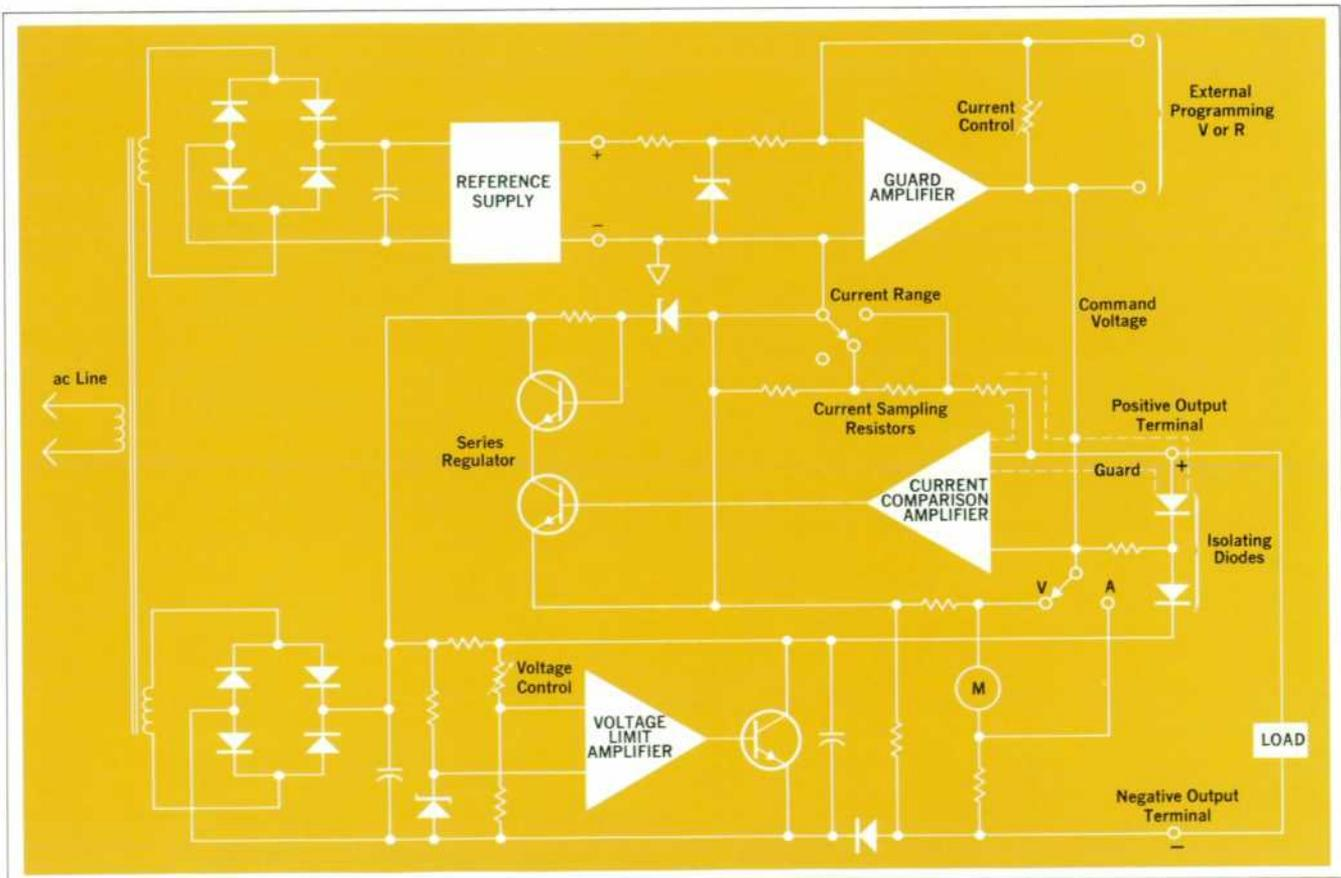
**Fig. 4.** Command voltage for current regulator comes from internal reference supply or from external programming voltage or resistance. Voltage-limit circuit quickly draws current away from load when load voltage exceeds voltage limits and isolating diodes turn on. High-gain regulator and absence of reactive elements in output give high output impedance, fast programming, and freedom from current overshoots.
