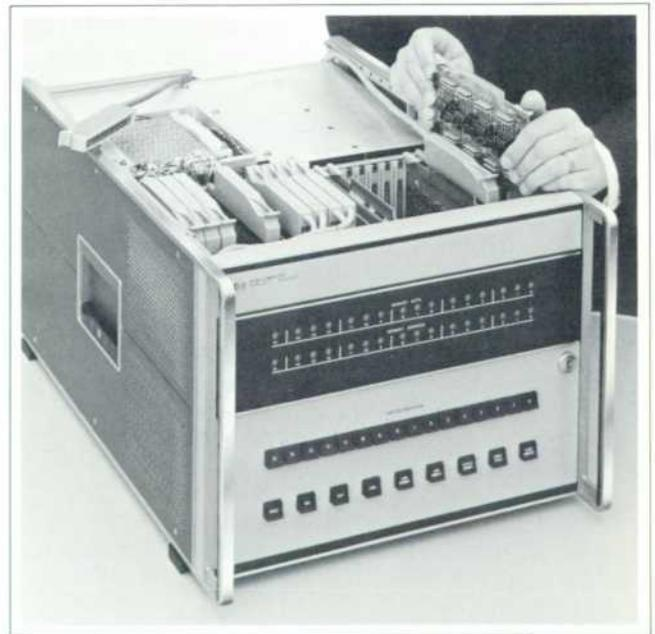
**Fig. 4.** Small general-purpose digital computers are being used more and more as controllers in automatic test systems because of the flexibility and versatility they offer. HP Models 2114A (shown here), 2115A, and 2116B are designed to accept interface cards which allow them to communicate with signal sources, measuring instruments, and peripherals.
