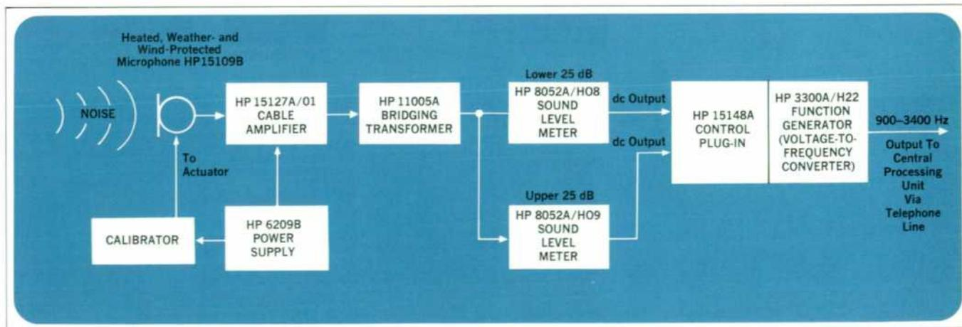
**Fig. 3.** Each noise monitoring terminal has a microphone system (not shown in Fig. 2) and two impulse sound-level meters. It can measure noise levels from 0 to 50 dB above a preset reference level (0 to 75 dB with options).
