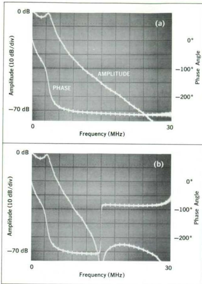
**Fig. 3.** A third order Chebyshev low-pass filter with 3 dB passband ripple and 4 MHz cutoff shows phase nonlinearity in the passband and the nearby stopband (a). The phase tends toward  $-270^\circ$  ( $-90^\circ$  per pole). The same filter (b) modified to produce a transmission zero at 15 MHz shows a characteristic phase shift of nearly  $+180^\circ$  at zero. The second transmission zero just beyond 30 MHz is caused by parasitics. Markers on these scope photos are 1 MHz.
