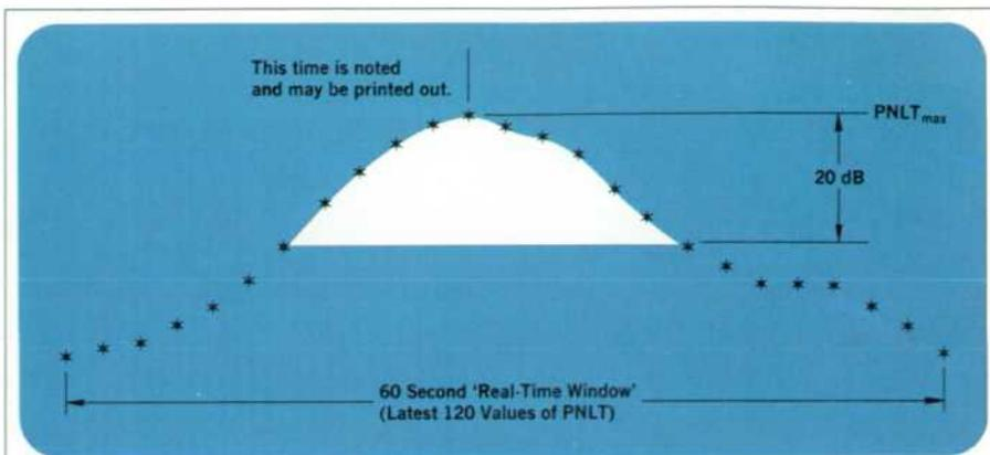
THIS PROGRAM PERFORMS A COMPUTATION ON READINGS OBTAINED FROM THE HP 8054A REAL TIME AUDIO SPECTRUM ANALYZER. THE PROCEDURE ADOPTED CONFORMS TO THE ISO RECOMMENDATIONS 507 FOR DESCRIBING AIRCRAFT NOISE AROUND AN AIRPORT.
