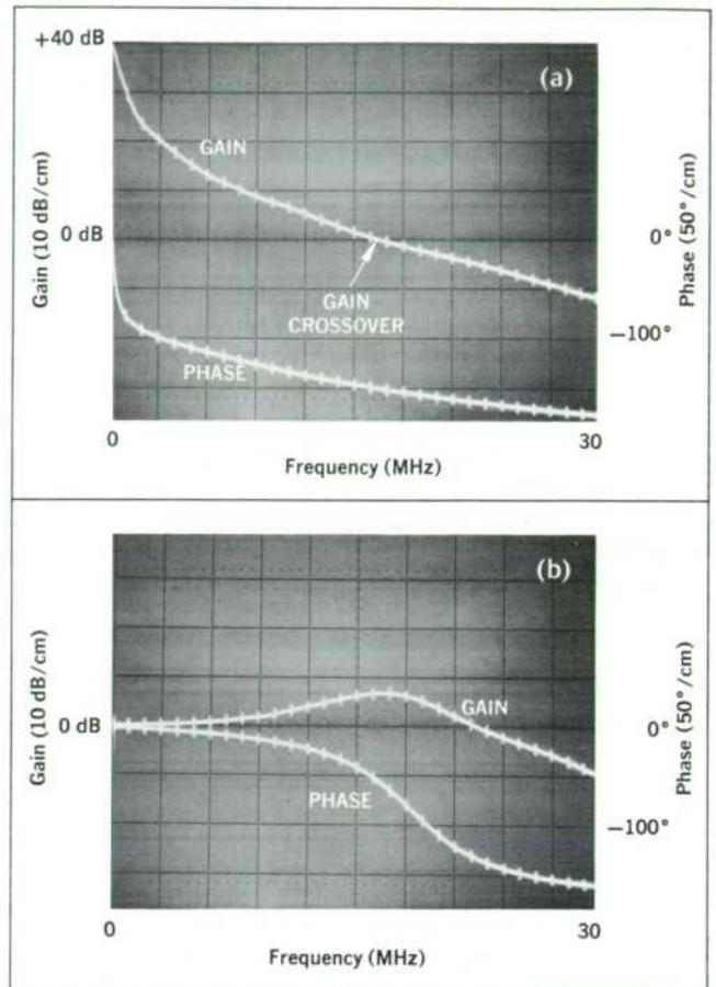
**Fig. 4.** Open loop characteristics of a video amplifier (a) shows a low-frequency gain of 40 dB, gain crossover at 16.5 MHz and a phase shift at gain crossover of  $150^\circ$ , giving a phase margin of  $30^\circ$ . With unity gain feedback (b) the amplifier shows about 6 dB of peaking.
