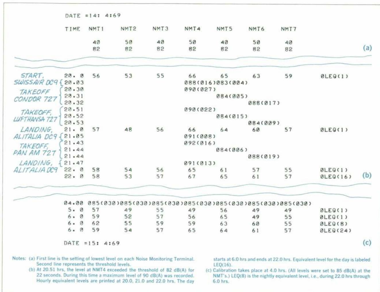
**Fig. 1.** Model 80500A Aircraft Noise Monitoring System continuously monitors the noise level at many points around an airport and indicates excess levels immediately so corrective action can be taken. This is a printout for the seven-point system at Stuttgart airport.
