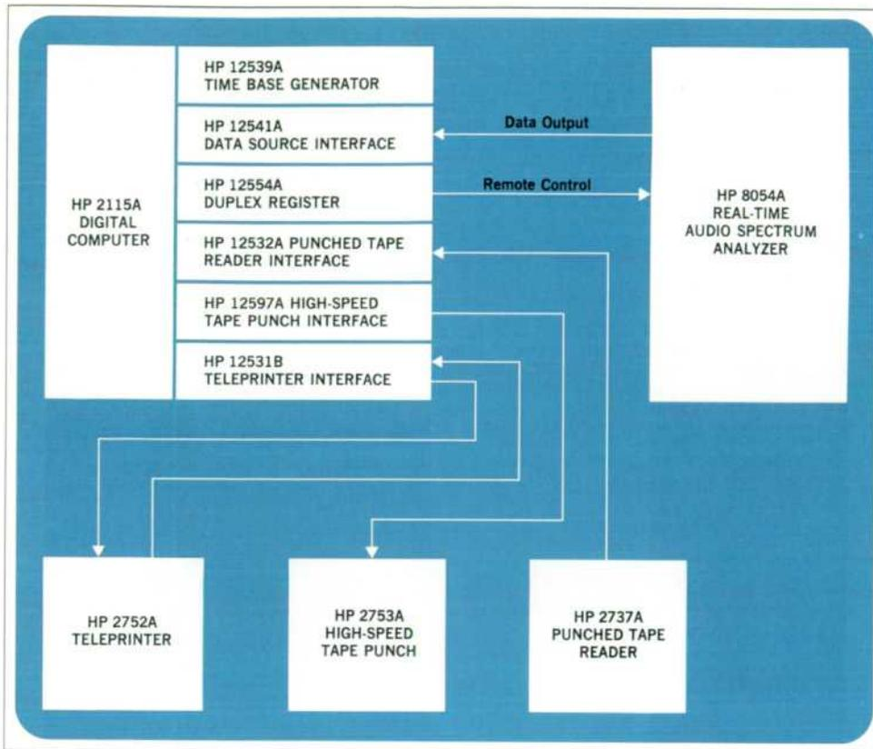
**Fig. 2.** The computer completely controls the analyzer's operation, even adjusting its range according to the input level. Additional peripherals or analyzers can be incorporated into the system simply by plugging standard interface cards into the computer.
