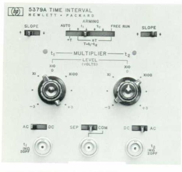
**Fig. 3.** Model 5379A Time-Interval Plug-in is used with the computing counter to measure time intervals with  $\pm 1$  ns accuracy and  $\pm 0.1$  ns resolution. Intervals down to zero can be measured, and if the stop pulse ( $t_2$  input) occurs before the start pulse ( $t_1$  input) the display will have a minus sign.
