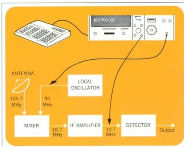
**Fig. 6.** This is an example of how the keyboard and the computing counter can work together to make measurements that would be awkward for conventional counters. The received signal at 105.7 MHz is too weak to be counted. A simple six-step program directs the counter to measure the 95 MHz LO frequency and the 10.7 MHz IF and add them to get the received frequency.
