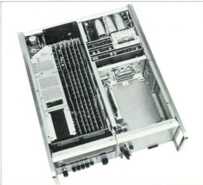
**Fig. 5.** Where to put 500 IC's, a 5 V, 10 A power supply, the crystal and interpolator ovens, and the other circuits was a problem that took six man-years to solve. All parts are easily removable for servicing.
