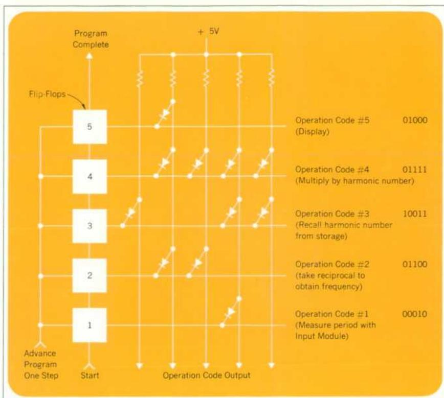
computing counter are all of the hard-wired read-only type, some made up of diode matrices (see Fig. 2) and others made up of gating networks. In addition to these internal programs, programs may be entered manually and stored in the accessory keyboard, or single steps may be executed manually using the keyboard.
