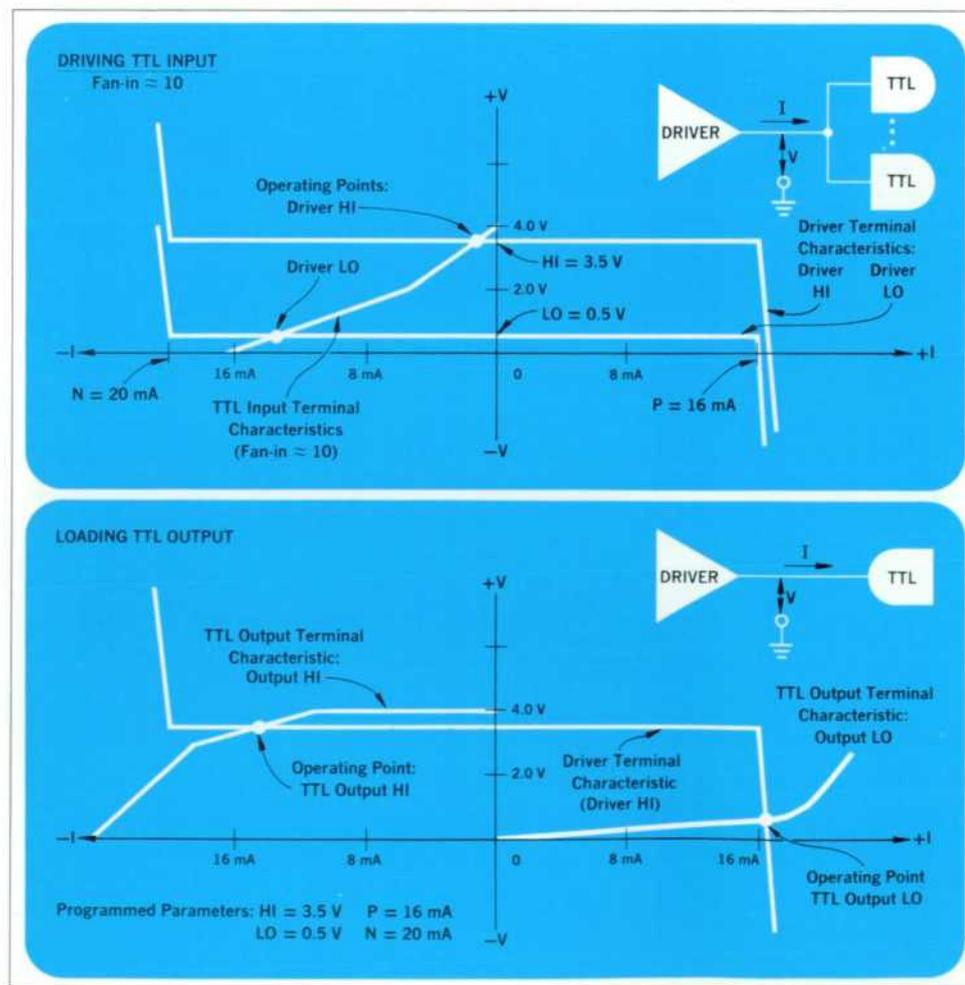
Fig. 4. The driver circuits can act as input generators, as loads, or as both simultaneously. Thus the system doesn't care whether a particular pin is an input pin or an output pin; the difference is important only in the test program. Here is how a driver circuit works with TTL logic.
