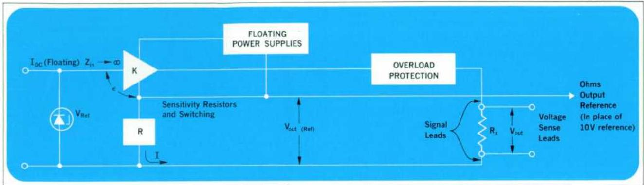
**Fig. 14.** Ohms measurements are made by taking the ratio of  $V_{out}$  to  $V_{out(Ref)}$ . Resistor  $R$  determines current  $I$  which also flows through  $R_x$ . Thus the ratio of the two voltages is the ratio of  $R_x$  to  $R$ . Amplifier error  $\epsilon$  and the magnitude of  $V_{ref}$  do not affect measurement accuracy.
