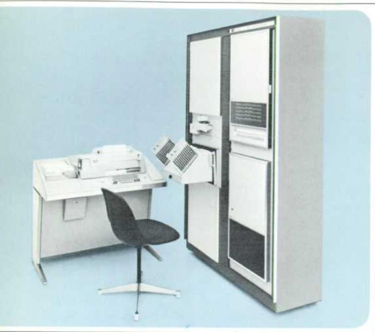
**Fig. 1.** Model 2060A Digital Logic Module Test System can give most production logic modules a thorough functional test in less than 30 seconds. It is programmed in AuTest, a special simplified language. Once programmed, it can be used by unskilled operators.
