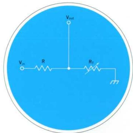
Fig. 8. To accurately determine the value of  $R_1$ , the ratio of  $V_{out}$  to  $V_{in}$  is more important than the absolute value of  $V_{out}$ . Accuracy is then independent of variations in  $V_{in}$ .
