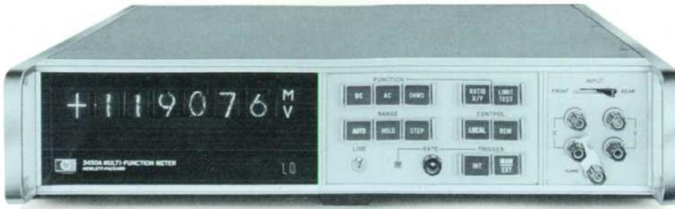
Fig. 4. Basically a five-digit integrating DVM, the HP Model 3450A measures dc voltage and voltage ratios. With plug-in options, measurement capabilities including ac, ohms, limit tests, digital output and remote control may be added.
