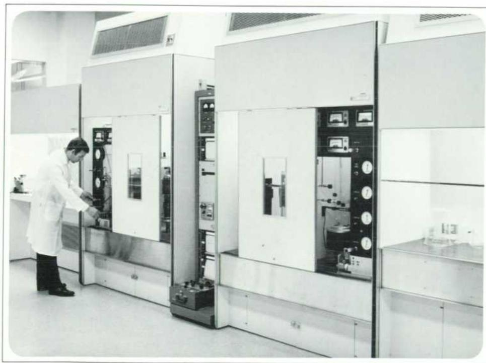
**Fig. 7.**  $Ga(As,P)$  wafers up to two inches in diameter are grown in this HP-designed vertical-flow, RF-heated, cold-wall, dual-reactor, vapor-phase epitaxial system. The light-emitting diodes are made from these wafers. All parts of the solid-state indicators except the case are made by HP.
