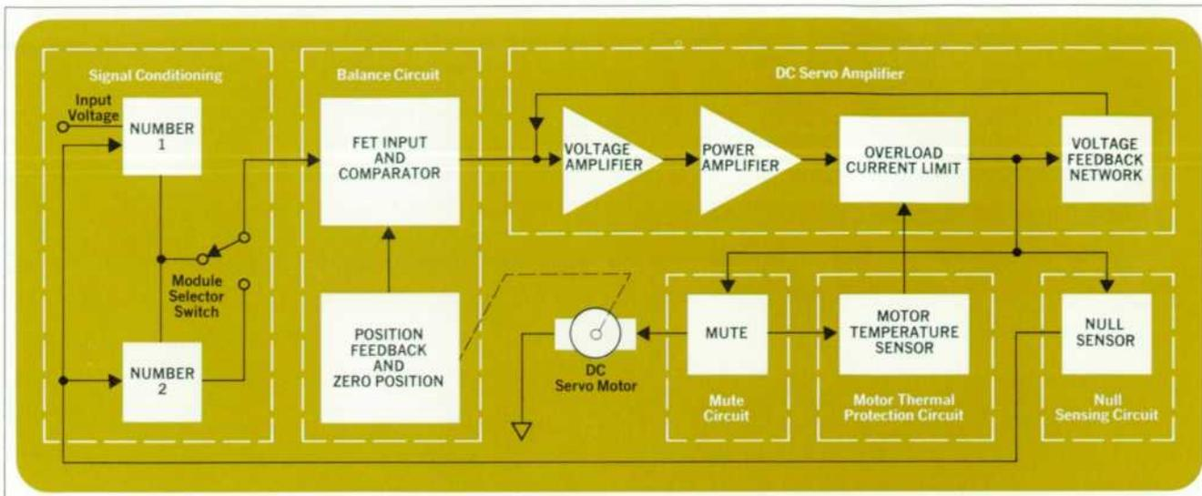
Fig. 4. Six functional blocks make up the Model 7004A main frame. Numbers 1 and 2 in the Signal Conditioning area are spaces for the plug-ins.
