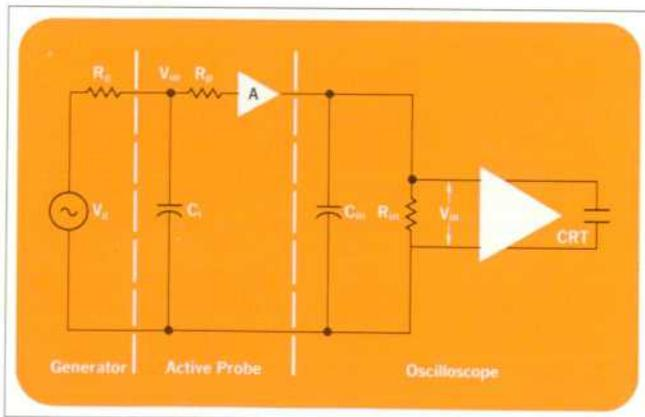
Fig. 5. Equivalent circuit of a typical active probe.
