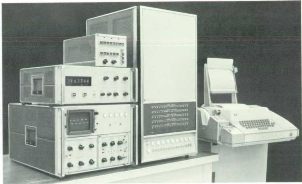
part of memory to another. The coupler can add or subtract two waveforms (to 24-bit precision) and return the result to memory. For more complex processing, the coupler interfaces the analyzer with a general-purpose digital computer.
