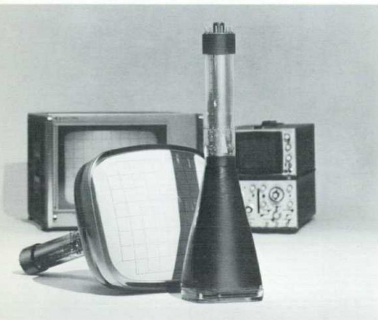
*A very large CRT display in a relatively short envelope (Model 1300A CRT, left) can be obtained by suitable design of the expansion mesh. Other engineering factors appropriate to specific applications may dictate an expansion mesh design to accommodate smaller displays.*
