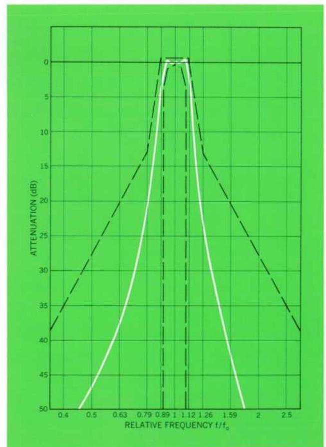
Fig. 6. Typical response curve for 1/3-octave filter used in loudness analyzer. Response is down more than 20 dB at center frequency of following filter, and down 60 dB at twice the center frequency. Dashed curves show tolerances allowed by international standards.
