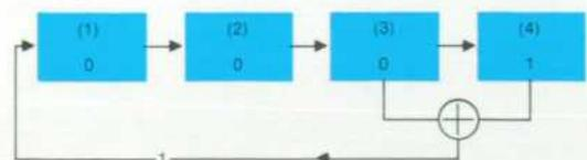
The fifteenth pulse restores the register to the initial state (1000), and thereafter the sequence repeats.
