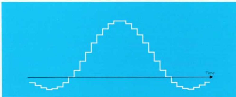
Fig. 13. Single-pulse response of digital filter is a discrete-step approximation to  $(\sin x/x)$ -shaped impulse response of ideal low-pass filter.
