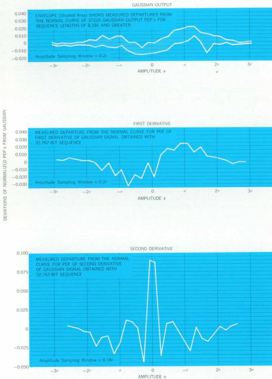
Fig. 17. Measured deviations from true Gaussian probability density function for noise generator 'Gaussian' output are less than about  $\pm 10\%$  for sequence lengths of 8191 and greater. First two derivatives are also reasonably Gaussian.
