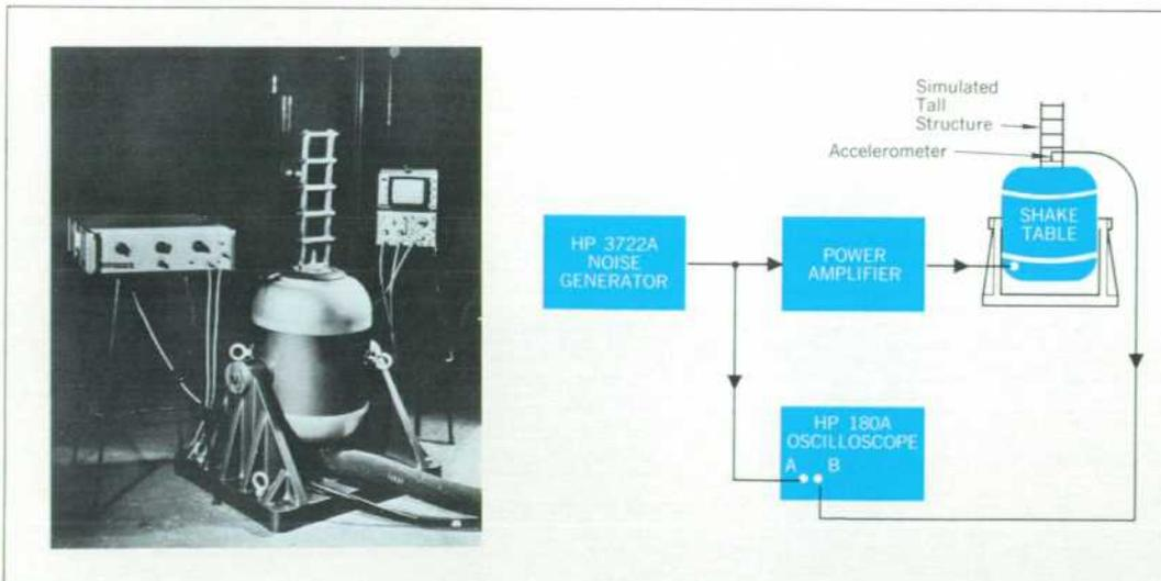
Fig. 1. Model simulation of tall structure. Noise-driven shake table simulates ground disturbances, and accelerometer measures structure's response.
