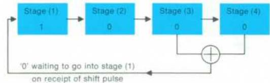
The modulo-two sum of the outputs from the last two stages is '0' (this can be written  $0 \oplus 0 = 0$ ). At the first shift pulse, the '1' in the first stage is transferred to the second, and is replaced by the '0' in the feedback line. This gives the pattern:
