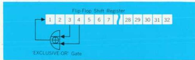
Fig. 8. Fifteen-bit pseudo-random binary sequence is generated by four stages of shift register with feedback.
