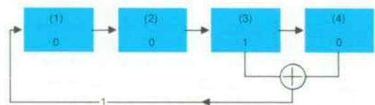
With this pattern, the outputs from the third and fourth stages are dissimilar — so the modulo-two sum is '1'. The '1' thus placed in the feedback line will enter the first stage on arrival of the next shift pulse.
