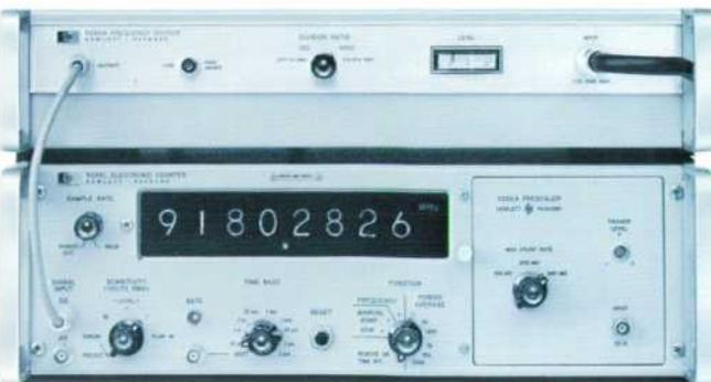
Fig. 1. Automatic Frequency Divider, *-hp-* Model 5260A, divides input frequencies between 0.3 GHz and 12.4 GHz by 100 or 1000 so they can be measured by a counter (counter shown is *-hp-* Model 5245L 50 MHz Counter). Divider operation is completely automatic except for selection of division ratio.
