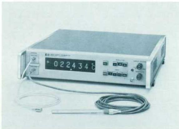
Fig. 4. A complete quartz thermometer system, the *-hp-* Model 2801A with two temperature sensing probes. With this system, the temperature of either probe or the difference between the temperatures of the two probes can be shown on the readout.
