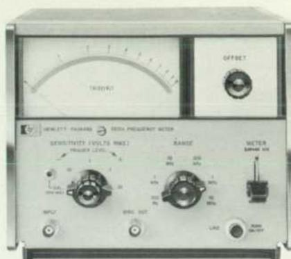
*Fig. 1. New -hp- Model 5210A Frequency Meter and FM Discriminator directly measures frequencies between 3 Hz and 10 MHz. Special log-linear meter scale can be read accurately within  $\pm 1\%$  of reading. Discriminator output is useful for measurements of instantaneous frequencies of FM signals, measurements that are impossible for most other frequency measuring devices.*
