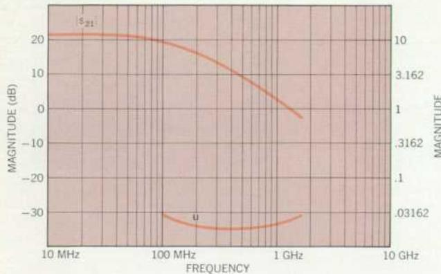
Fig. 5. Top curve:  $|s_{21}|$  from Fig. 4 replotted on logarithmic frequency scale. Data below 100 MHz measured with *hp-8405A* Vector Voltmeter. Bottom curve: unilateral figure of merit, calculated from *s* parameters (see text).
