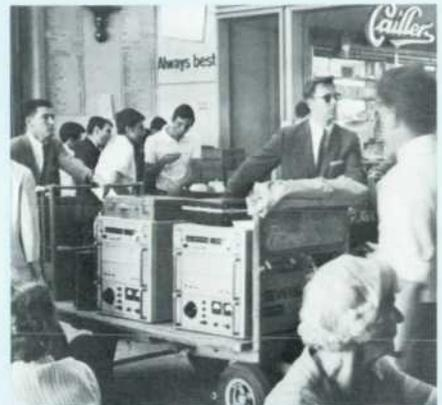
*No matter what the mode of transport, flying clocks were kept in continuous operation throughout entire trip. Clocks were powered by internal batteries when ac line power or auto or airplane electrical power was not available. -hp- engineers Lee Bodily (right) and Ron Hyatt (left) transfer clocks at Geneva airport.*
