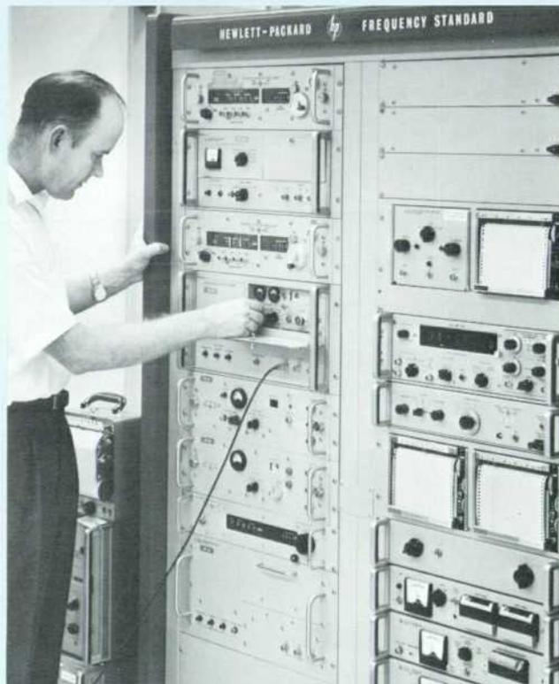
The clock mechanism immediately above the Cesium Standard integrates the Cesium Standard output to show any accumulated phase error.
