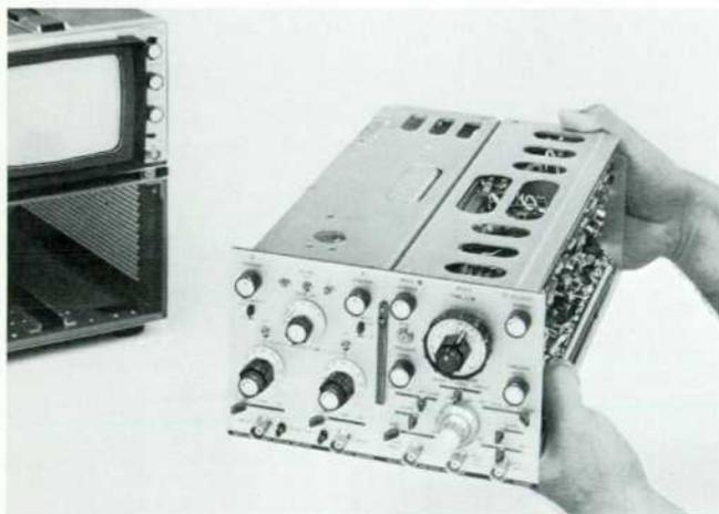
Fig. 13. Plug-ins are connected mechanically and electrically before insertion into the cabinet.
