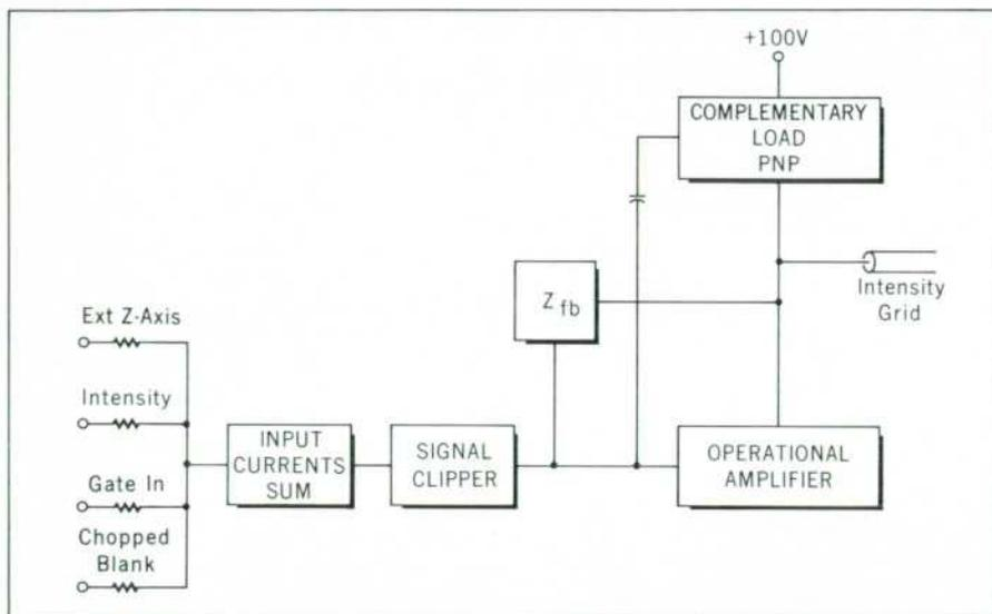
Fig. 12. Various inputs to the gate amplifier are converted to currents and added in a common-base amplifier.
