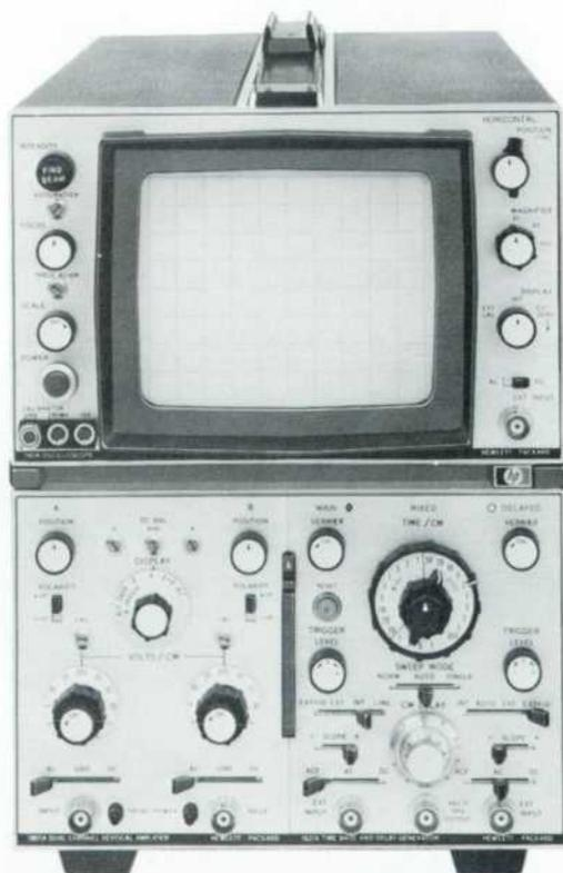
Fig. 3. The front panel of the oscilloscope, shown here  $\frac{3}{8}$  actual size, is slightly shorter than this page height and slightly narrower than this page width. Controls are clearly marked and arranged so they are not obscured by cables. Plug-ins are in the lower half of this cabinet version, with CRT beam controls and horizontal amplifier controls in the upper half.
