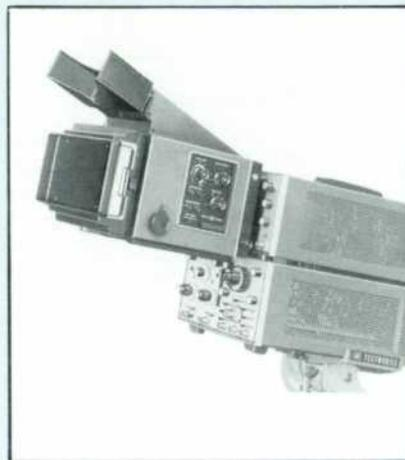
slip feet were not placed on the back so that, when the scope is being used face up, it will slide if bumped rather than tip. These rear feet are high enough so that cables run free underneath.
