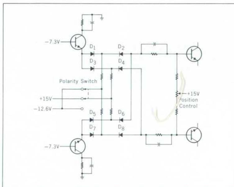
Fig. 6. Polarity of the input to the vertical amplifiers is switched by switching diode gates. In the 'up' or + position, diodes  $D_1$ ,  $D_2$ ,  $D_3$  and  $D_4$  are turned on while  $D_5$ ,  $D_6$ ,  $D_7$  and  $D_8$  are reversed biased. The signal path is across  $D_1$ ,  $D_3$ , and  $D_7$ ,  $D_5$ . Reversing polarity reverses the bias.
