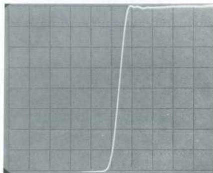
Fig. 8. A pulse with less than 7 ns rise time illustrates the bandwidth capabilities of the scope.
